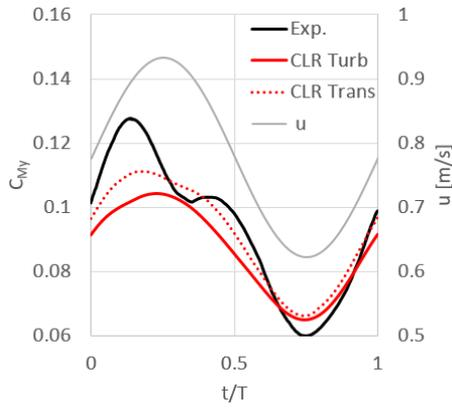
Fig. 13. Measured data [7] and CFD results for the time-dependent out-of-plane blade root bending moment over the oscillating cycle at  $\omega=73$  RPM, mean  $\lambda=3.6$ ,  $\mu=0.2$  and  $f=0.5$  Hz.
