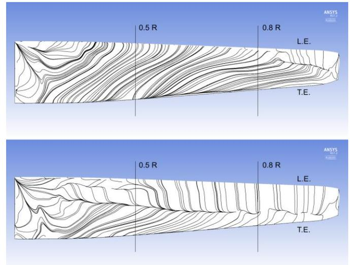
Fig. 7. Computed wall shear stress lines on the SS of the blade of the towing tank TCT at  $\omega=73$  RPM at  $\lambda=2.81$  (top plot) and  $\lambda=3.6$  (bottom plot).
