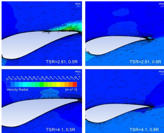
Fig. 16. Computed velocity vectors and contours of radial velocity components at  $\omega=96$  RPM and  $Re_c=8.4$  million. Top left: cylindrical slice at  $0.5R$  and  $\lambda=2.81$ . Top right: cylindrical slice at  $0.8R$  and  $\lambda=2.81$ . Bottom left: cylindrical slice at  $0.5R$  and  $\lambda=4.1$ . Bottom right: cylindrical slice at  $0.8R$  and  $\lambda=4.1$ .
