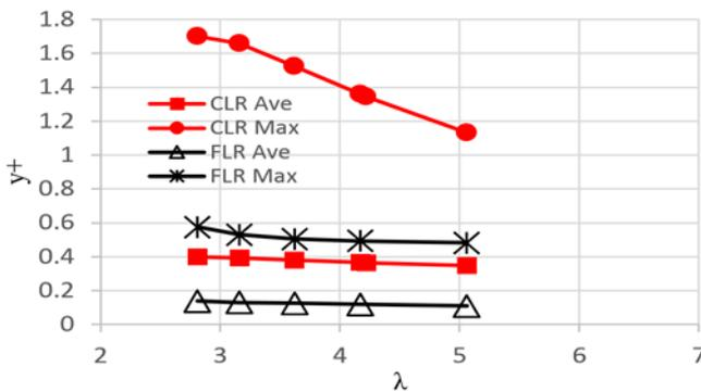
Fig. 8. Minimum and averaged  $y^+$  on the SS of the blade of the towing tank TCT against TSR at  $\omega=73$  RPM.
