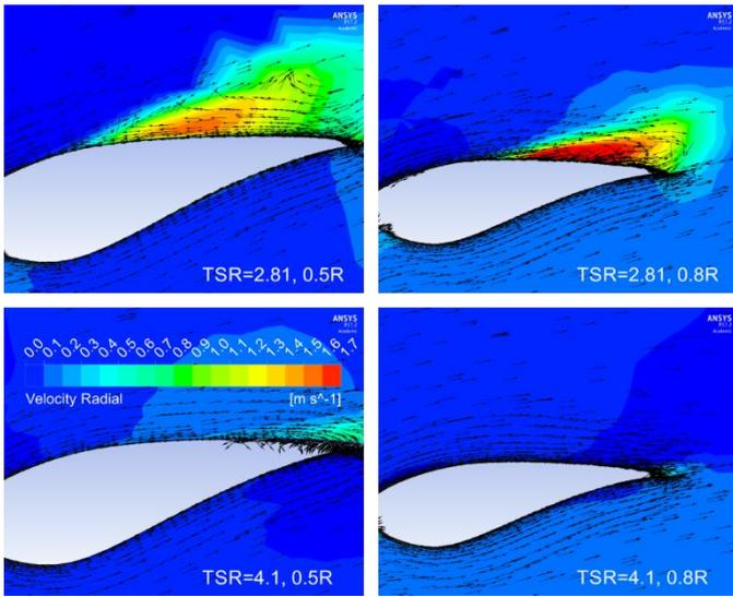
Fig. 10. Computed velocity vectors and contours of radial velocity components of towing tank TCT at  $\omega=96$  RPM. Top left: cylindrical slice at  $0.5R$  and  $\lambda=2.81$ . Top right: cylindrical slice at  $0.8R$  and  $\lambda=2.81$ . Bottom left: cylindrical slice at  $0.5R$  and  $\lambda=4.1$ . Bottom right: cylindrical slice at  $0.8R$  and  $\lambda=4.1$ .
