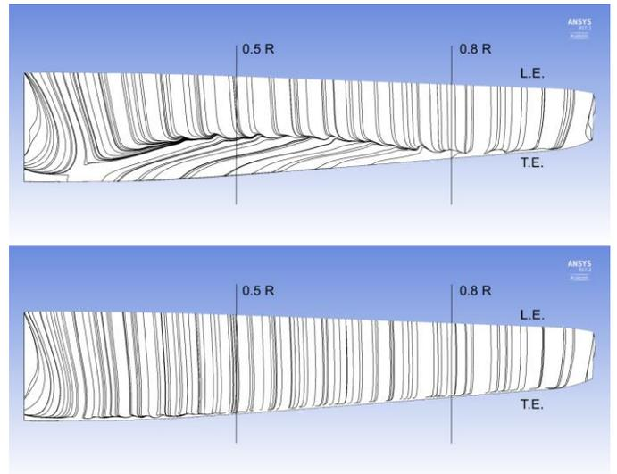
Fig. 17. Computed wall shear stress lines on the SS of the blade of the towing tank TCT at  $\omega=96$  RPM and  $Re_c=8.4$  million. Top: wall shear stress lines at  $\lambda=2.81$ . Bottom: wall shear stress lines at  $\lambda=4.1$ .
