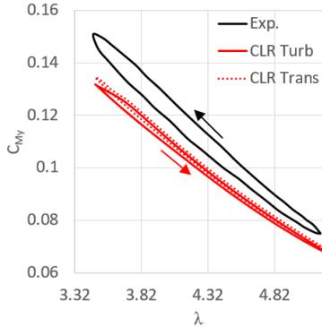
Fig. 14. Measured data [7] and CFD results for the time-dependent out-of-plane blade root bending moment against instantaneous TSR at  $\omega=96$  RPM, mean  $\lambda=4.1$ ,  $\mu=0.2$  and  $f=0.5$  Hz.
