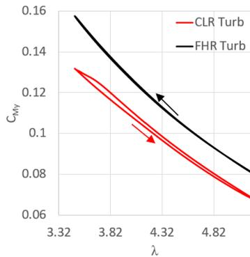
Fig. 19. Comparison of CFD results for the time-dependent low- and high--Reynolds number out-of-plane blade root bending moment against instantaneous TSR at  $\omega=96$  RPM, mean  $\lambda=4.1$ ,  $\mu=0.2$  and  $f=0.5$  Hz. ('CLR': coarse grid for  $Re_c=116,000$  analysis; 'FHR': fine grid for  $Re_c=8.4$  million analysis; 'Turb': fully turbulent simulation).
