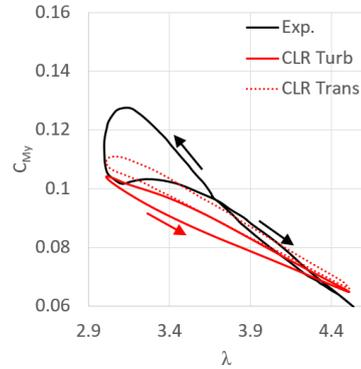
Fig. 12. Measured data [7] and CFD results for the time-dependent out-of-plane blade root bending moment against instantaneous TSR at  $\omega=73$  RPM, mean  $\lambda=3.6$ ,  $\mu=0.2$  and  $f=0.5$  Hz.
