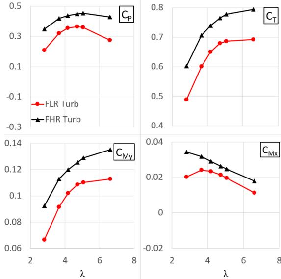
Fig. 15. Low- and high-Reynolds number CFD results for different TSRs at  $\omega=96$  RPM ('FLR': fine grid for  $Re_c=116,000$  analysis; 'FHR': fine grid for  $Re_c=8.4$  million analysis. 'Turb': fully turbulent analysis). Top left: power coefficient; top right: thrust coefficient; bottom left: out-of-plane root bending moment; bottom right: in-plane root bending moment.
