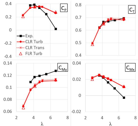
Fig. 9. Measured data [7] and CFD results for different tip-speed ratios at  $\omega=96$  RPM ('CLR' and 'FLR' denote coarse and fine grid respectively, 'Turb' denotes fully turbulent simulation, and 'Trans' denotes transitional simulation). Top left: power coefficient; top right: thrust coefficient; bottom left: out-of-plane root bending moment; bottom right: in-plane root bending moment.
