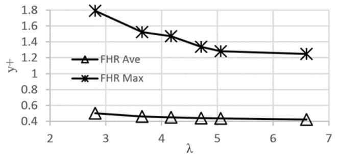
Fig. 18. Minimum and averaged  $y^+$  on the SS of the blade of the towing tank TCT against TSR at  $\omega=96$  RPM and  $Re_c=8.4$  million.
