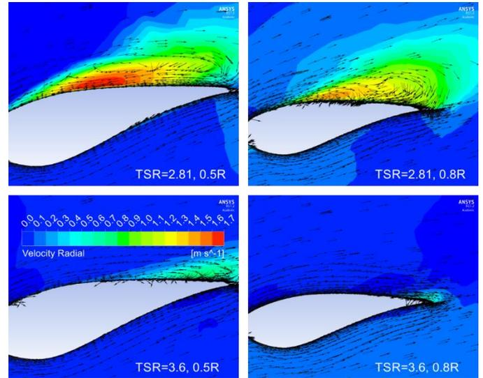
Fig. 6. Computed velocity vectors and contours of radial velocity components of towing tank TCT at  $\omega=73$  RPM. Top left: cylindrical slice at 0.5R and  $\lambda=2.81$ . Top right: cylindrical slice at 0.8R and  $\lambda=2.81$ . Bottom left: cylindrical slice at 0.5R and  $\lambda=3.6$ . Bottom right: cylindrical slice at 0.8R and  $\lambda=3.6$ .
