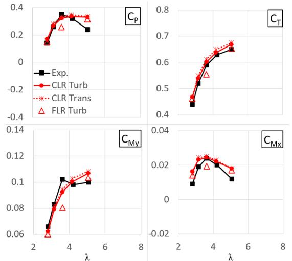
Fig. 5. Measured data [7] and CFD results for different TSRs at  $\omega=73$  RPM ('CLR' and 'FLR' denote coarse and fine grid respectively, 'Turb' denotes fully turbulent simulation, and 'Trans' denotes transitional simulation). Top left: power coefficient; top right: thrust coefficient; bottom left: out-of-plane root bending moment; bottom right: in-plane root bending moment.
