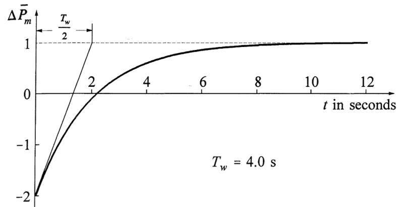
Fig. 6.1 Hydraulic turbine mechanical power output response to gate position step change [KBL94].
