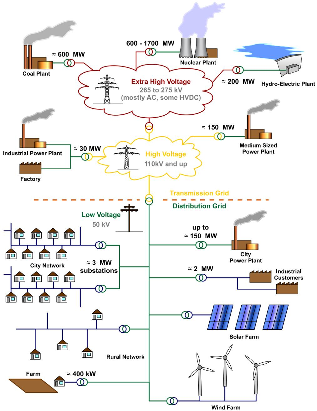
Fig. 2.2 General layout of the electricity networks in the USA [ele].
