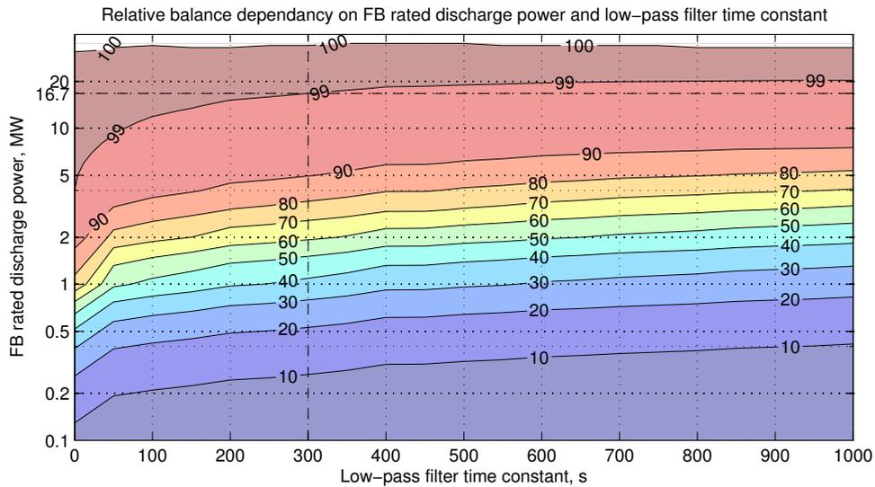
Fig. B.11 Relative balance dependency on FB rated discharge and LPF time constant.
