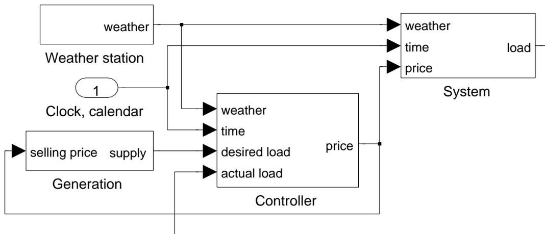
Fig. 2.8 System block diagram.
