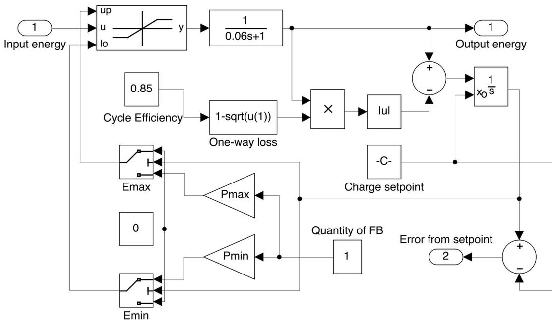
Fig. B.4 The structure of the flow battery model
