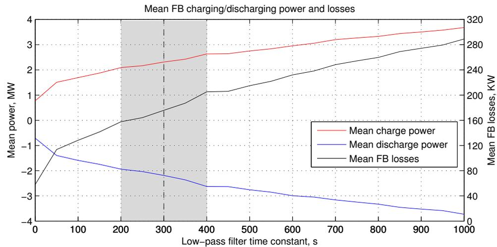
Fig. B.7 Mean FB charging/discharging power and losses
