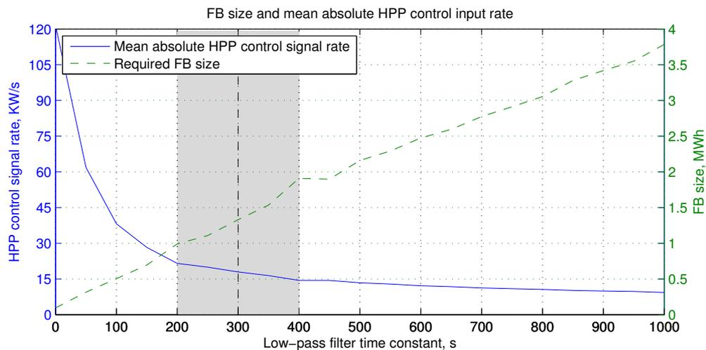
Fig. B.6 FB capacity and mean absolute HPP control input rate
