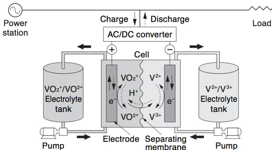
Fig. 6.5 Principle and configuration of a flow battery [Shi11].
