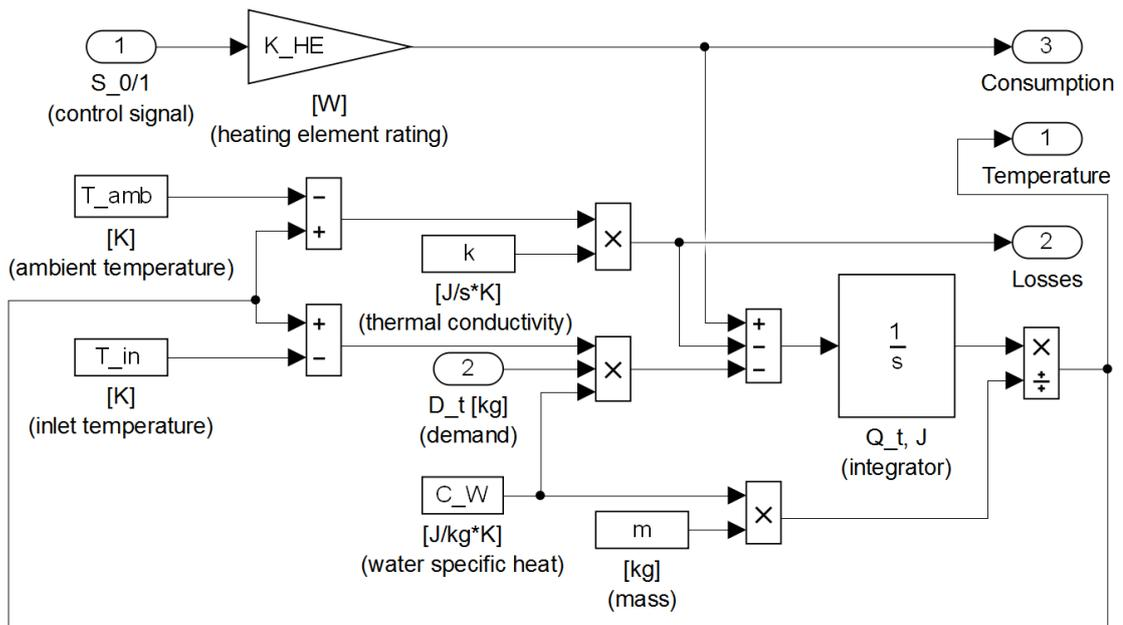
Fig. 5.2 Thermal water heater block diagram model.
