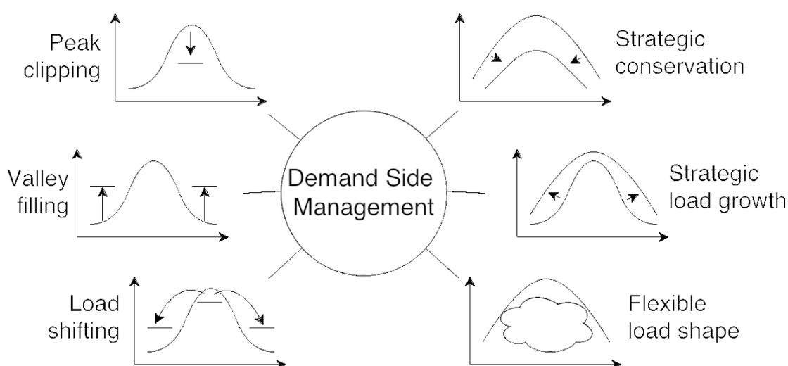
Fig. 2.5 Basic load shaping techniques [Gel85].
