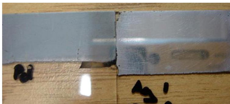
Fig. 4 Pd (left) and Ag (right) deposited by PIED onto the m-TiO 2 sensitised area of quartz slides.
