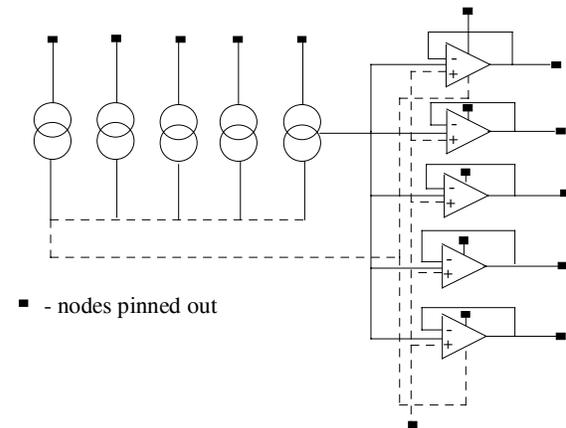
Figure 6: Schematic diagram of current reference chip cells
