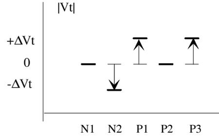
Figure 4: Parameter changes necessary for maximal current offset
