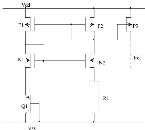
Figure 1: Schematic of current reference cell ( $i_{ref}$ )
