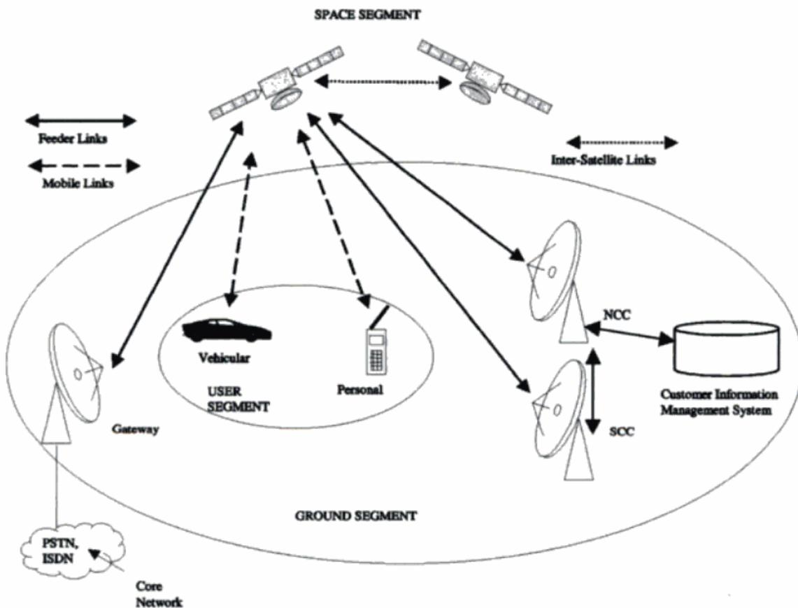
Figure 2 : Satellite Network Architecture [16]
