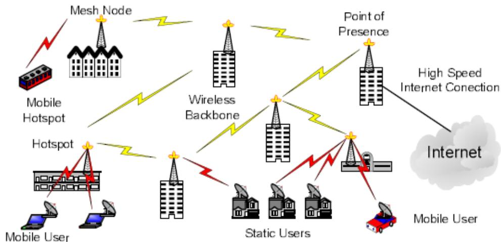
Figure 4 : WiMAX MESH Topology
