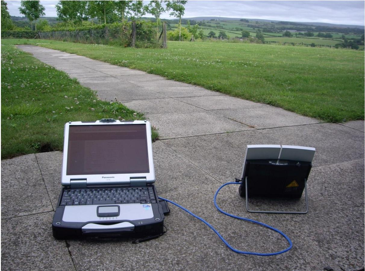
Figure 16 : Outdoors network tests of the Explorer 500 using a Panasonic Toughbook
