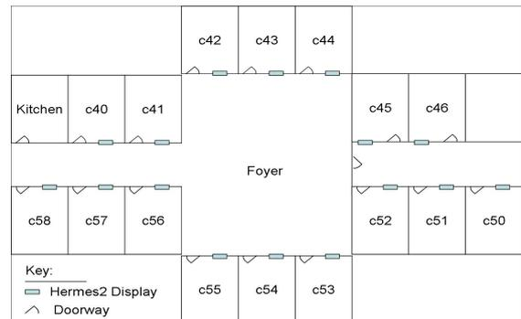
**Figure 3 – layout of a specific region of the Computing Department in Infolab showing offices (c42, c43, etc.) and the Hermes2 displays situated adjacent to doorways**
