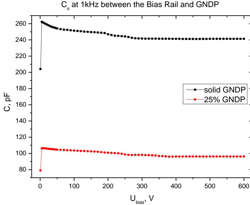
Fig.1 Capacitance between the Bias Rail and GNDP.
