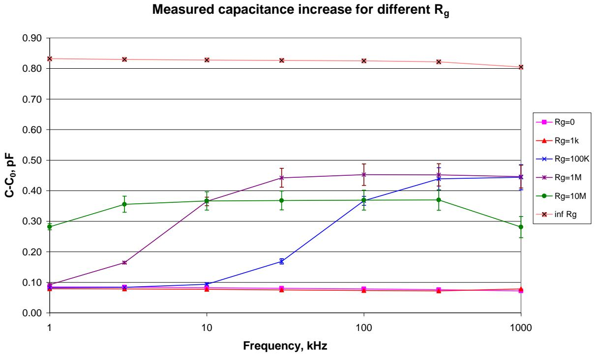
Fig.2 Additional to  $C_0$  capacitance vs. frequency for different  $R_g$ .
