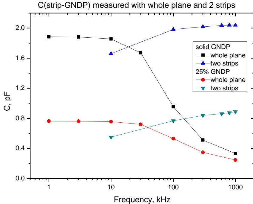
Fig.3. Frequency dependence of the  $C_g$  values for two sensors and two methods.
