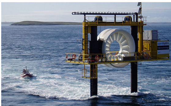
OpenHydro tidal turbine. Image from http://www.openhydro.com/
