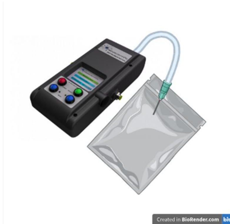
Fig.10. Representative visualisation of VOC sampling using portable VOC analyser as described.
