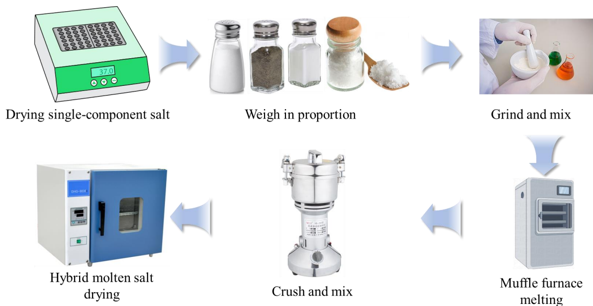
Fig. 3. Preparation method of mixed molten salt.
