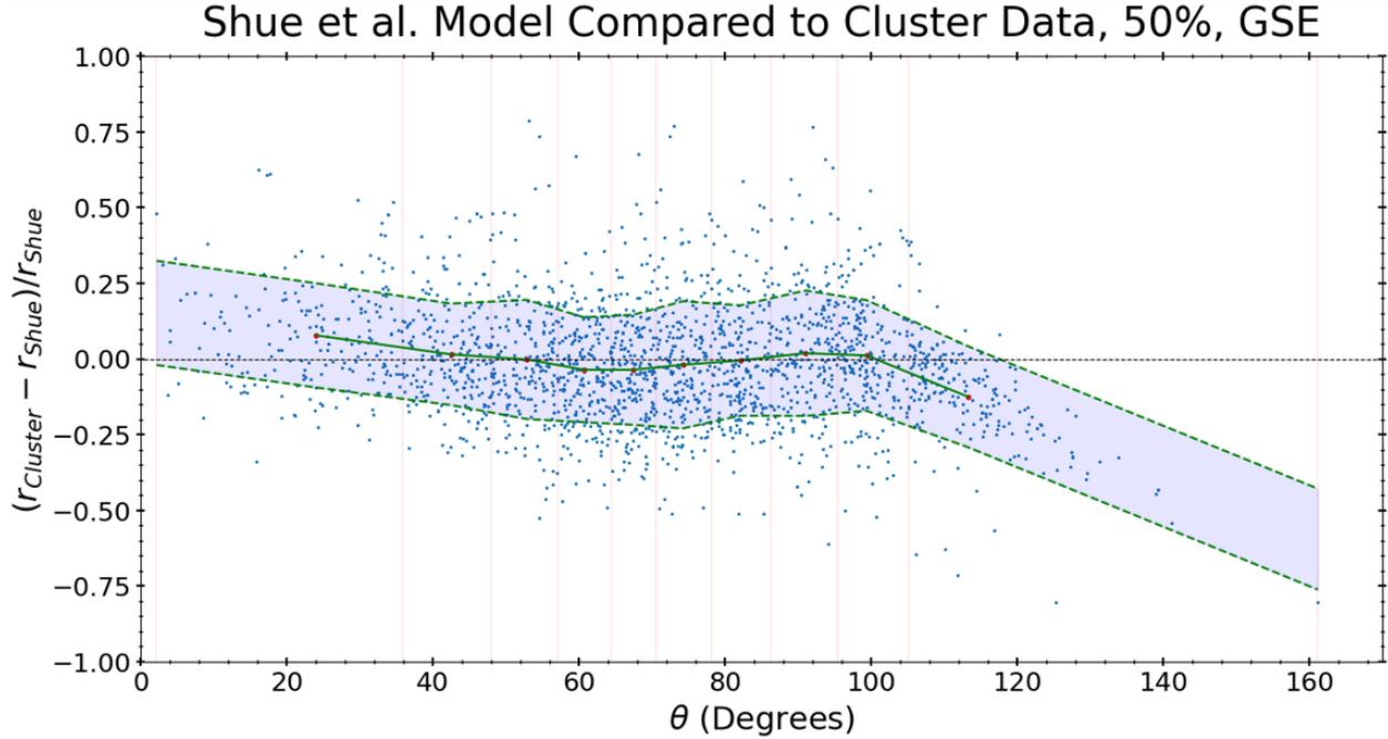
Figure 3.6: Comparison between the Cluster data and the Shue model r values as angle \theta increases. This is for shortest 50% of magnetopause crossings in GSE coordinates. Every 10% of the data, as the \theta value increases, is binned with the averages and standard deviations of these bins calculated and plotted. This gives the average line plotted in green with red points, and the standard deviation above and below the average plotted with the green dashed lines, with the blue shaded region between
