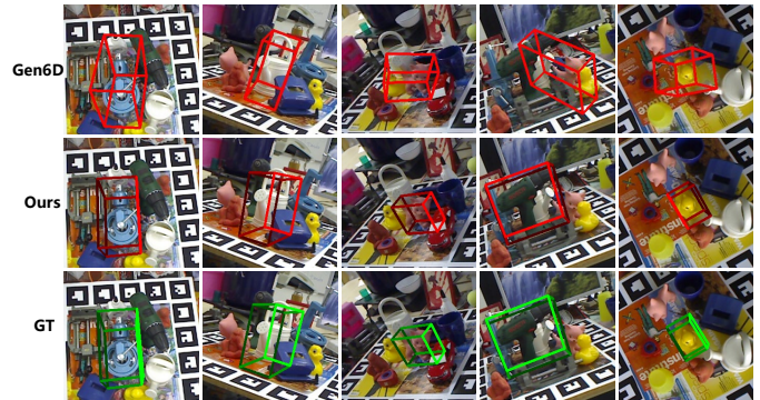
Fig. 5. The qualitative comparison results on the LineMod dataset [89] are presented, visualizing the outputs of Gen6D [69], our SinRef-6D, and ground truth from top to bottom.
