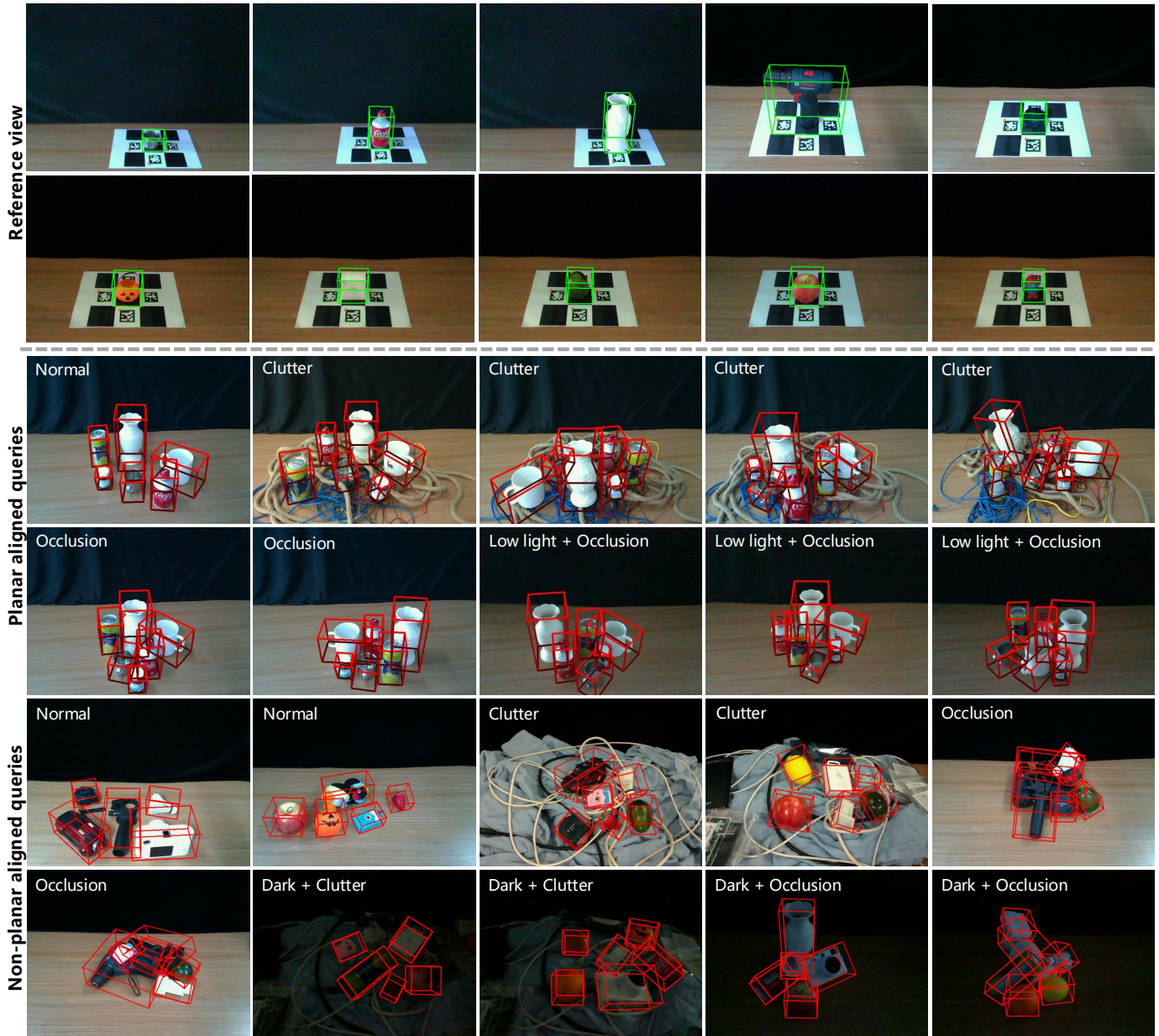
Fig. 8. Qualitative results on real-world robotic grasping scenarios. Top two rows : Single reference view capture and annotation from the robotic manipulation viewpoint for several unseen objects. Middle two rows : Unseen object 6-DoF pose estimation in planar aligned query views. Bottom two rows : Unseen object 6-DoF pose estimation in non-planar aligned query views. These include some challenging scenes commonly encountered in robotic grasping, including clutter, occlusion, low light, and dark conditions.
