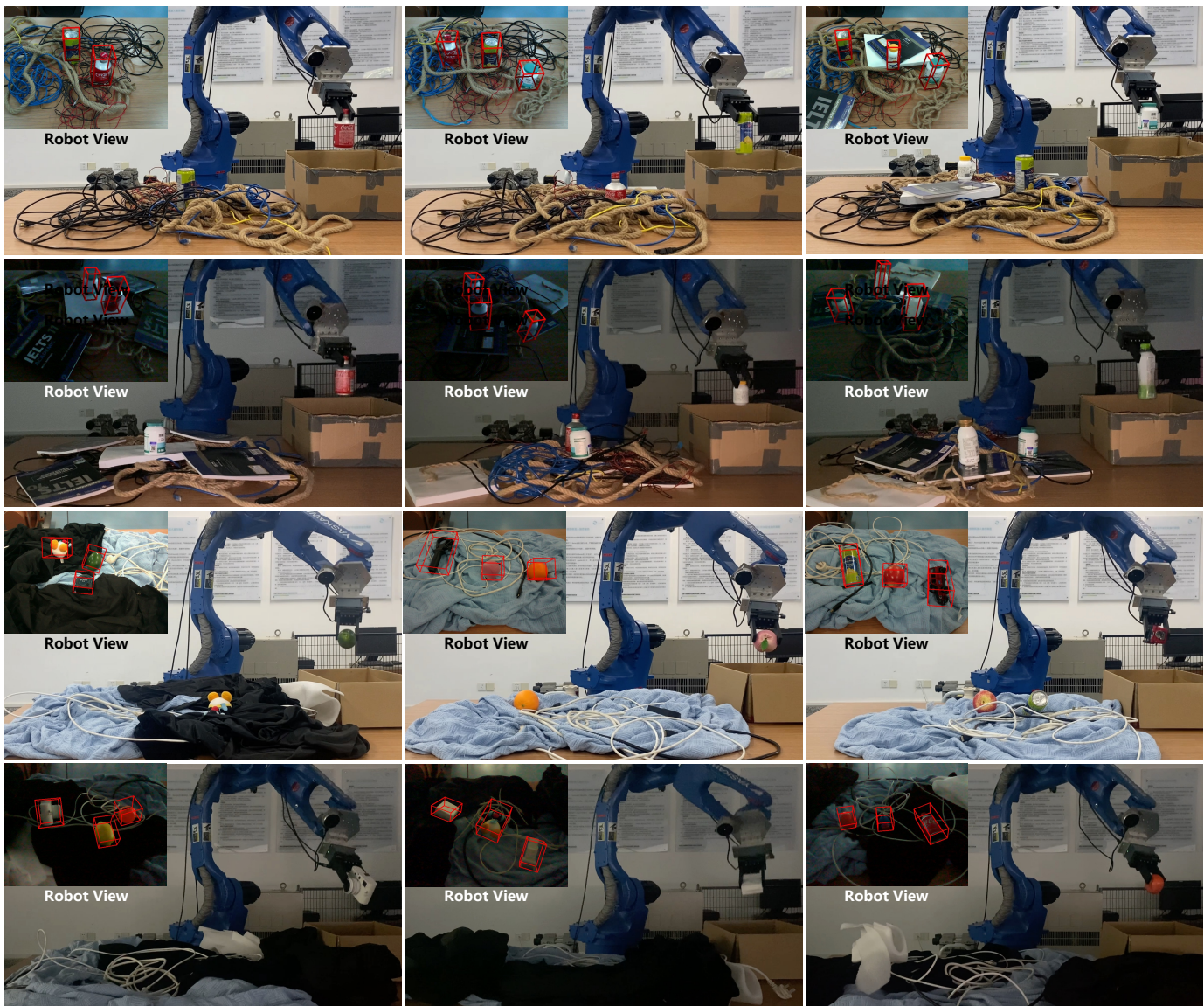
Fig. 9. Real-world robotic grasping visualizations. The top two rows and the bottom two rows represent planar aligned and non-planar aligned object grasping, respectively. These scenes contain clutter and low light. The top-left corner in each image shows the estimated 6-DoF poses of the unseen objects from the robotic manipulation viewpoint. The complete grasping video can be seen through our project homepage .
