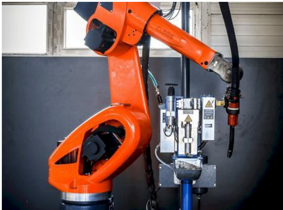
Figure 2. Six-axis CLOOS QRC 350 robotic welding system used in this research, source: https://www.exapro.com/cloos-qrc-350-qirox-p250516184/ (assessed 25th November 2025)
