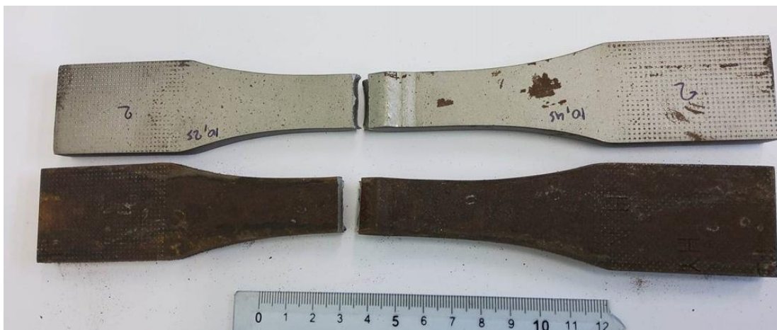
Figure 24: Non-corroded (top) and corroded (bottom) specimens after the fatigue test.
