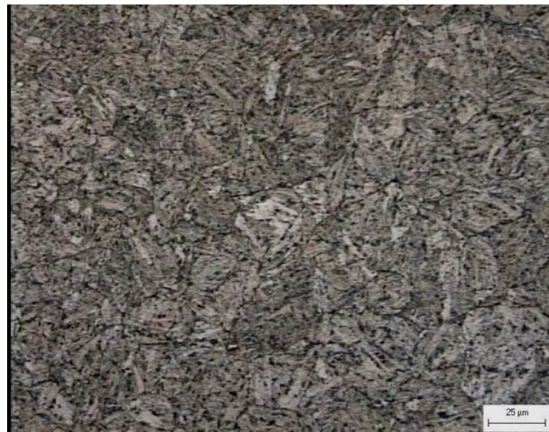
Figure 12: Bainitic phase in the HAZ region of HY 100 welded steel specimen.
