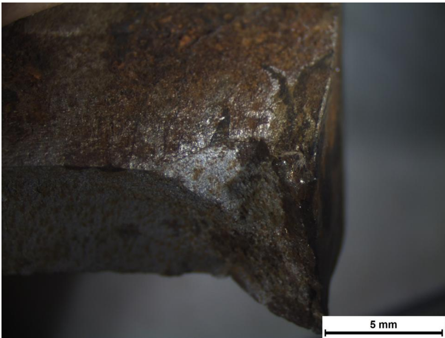
Figure 33: Corroded fracture surface of S355J2+N material
