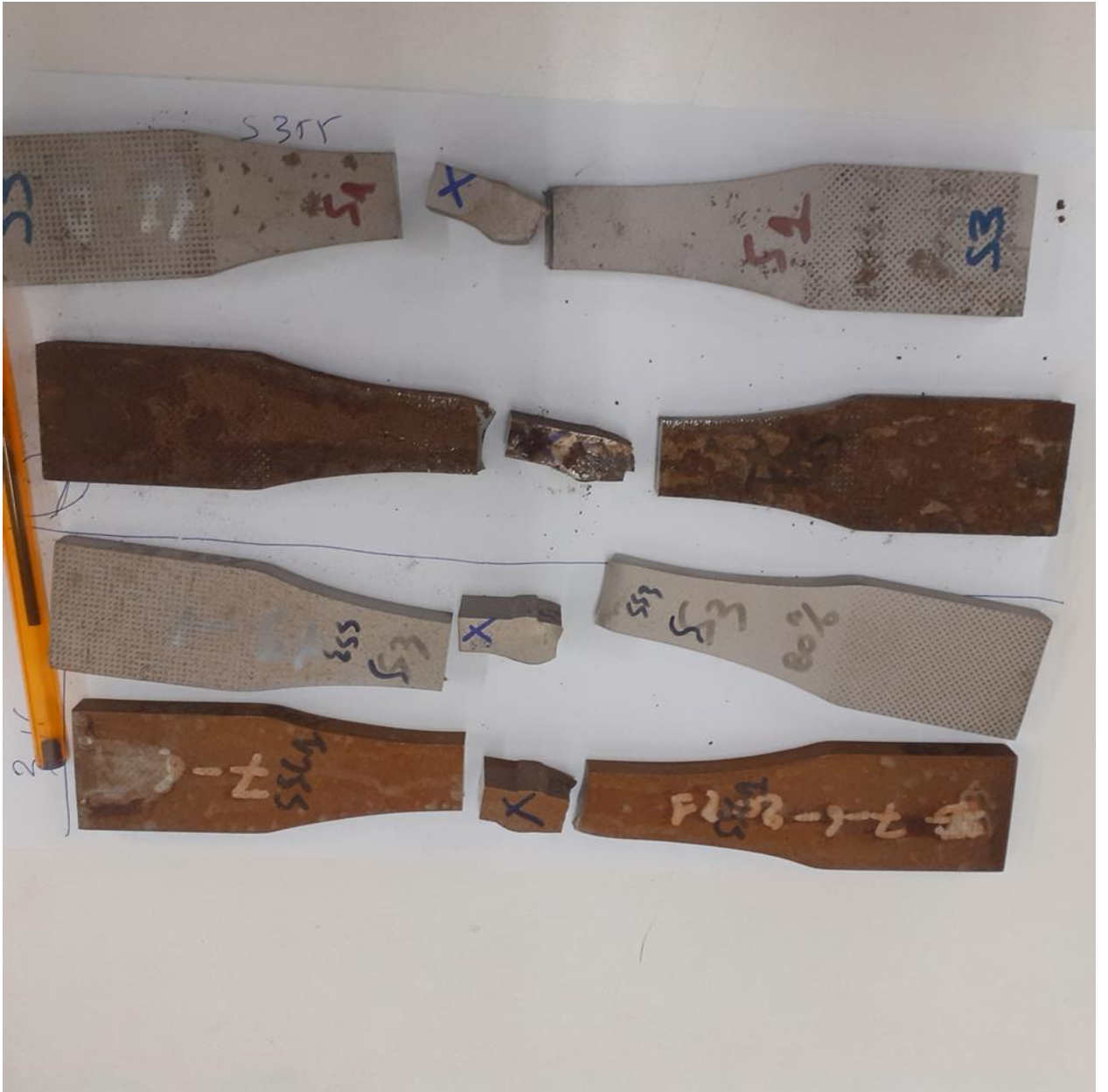
Figure 26: Non-corroded and corroded samples for two materials. X: indicates surfaces to be subjected in metallographic preparation (grinding, polishing, and etching).
