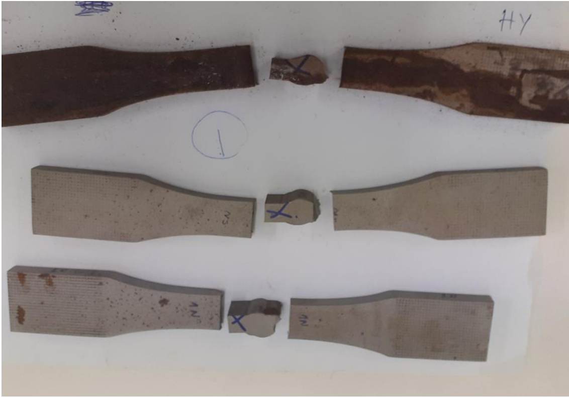
Figure 25: Corroded and non-corroded samples for HY 100. X: indicates surfaces to be subjected in metallographic preparation (grinding, polishing, and etching).
