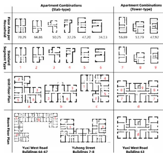
Figure 4-7. Formation of Residential Planes at the Beginning of the Construction of Zhengzhou No. 3 State-Run Cotton Textile Factory(modal grid method)(Zhou & Liu, 2022)
