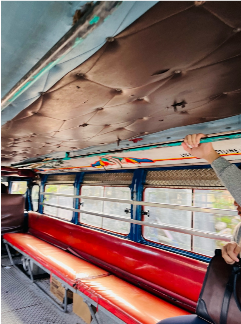
Figure 4.2.2 Bench-type seating and handlebars on both sides for passengers
