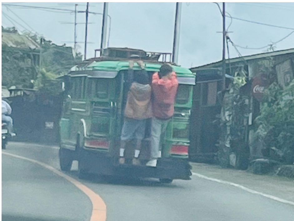
Figure 4.2.3 Passengers hanging on to an estribo on the jeepney's rear entrance
