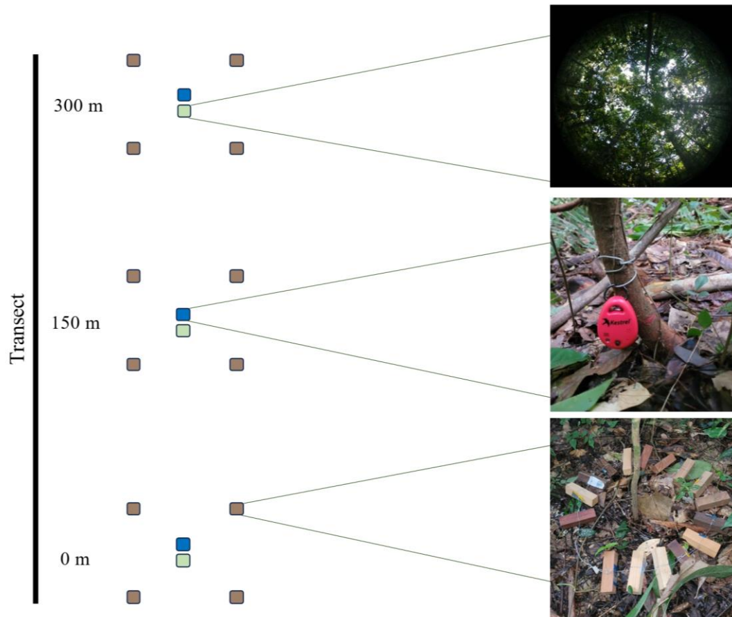
828 Fig. 1. Experimental sampling design. In each of the 18 sampled transects, we established three 829 sampling points, located at 0, 150 and 300 m. In each sampling point we installed four collars 830 (brown squares) and a microclimate data logger, which registered both temperature and relative 831 humidity (blue square). Hemispherical photographs were taken monthly at each sample point to 832 quantify canopy openness (green squares).
