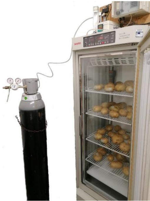
Figure 3.2 High-CO 2 longitudinal storage system comprising a Sanyo controlled environment cabinet (Sanyo), CO 2 vapour withdrawal cylinder, valve control system and secondary CO 2 meter.
