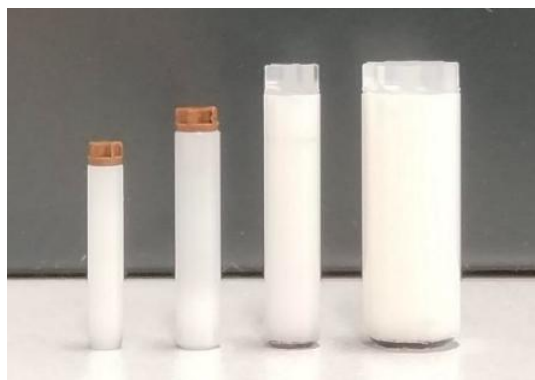
Figure 3.15: Examples of rotors used for NMR experiments. Outer diameters are 2.5, 3.2, 4 and 7 mm, left to right.
