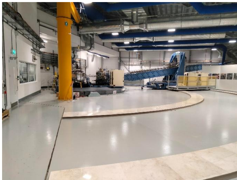
Figure 3.35: The RIXS spectrometer hall for the I21 beamline at Diamond Light Source. The blue detector arm is set to 90°.
