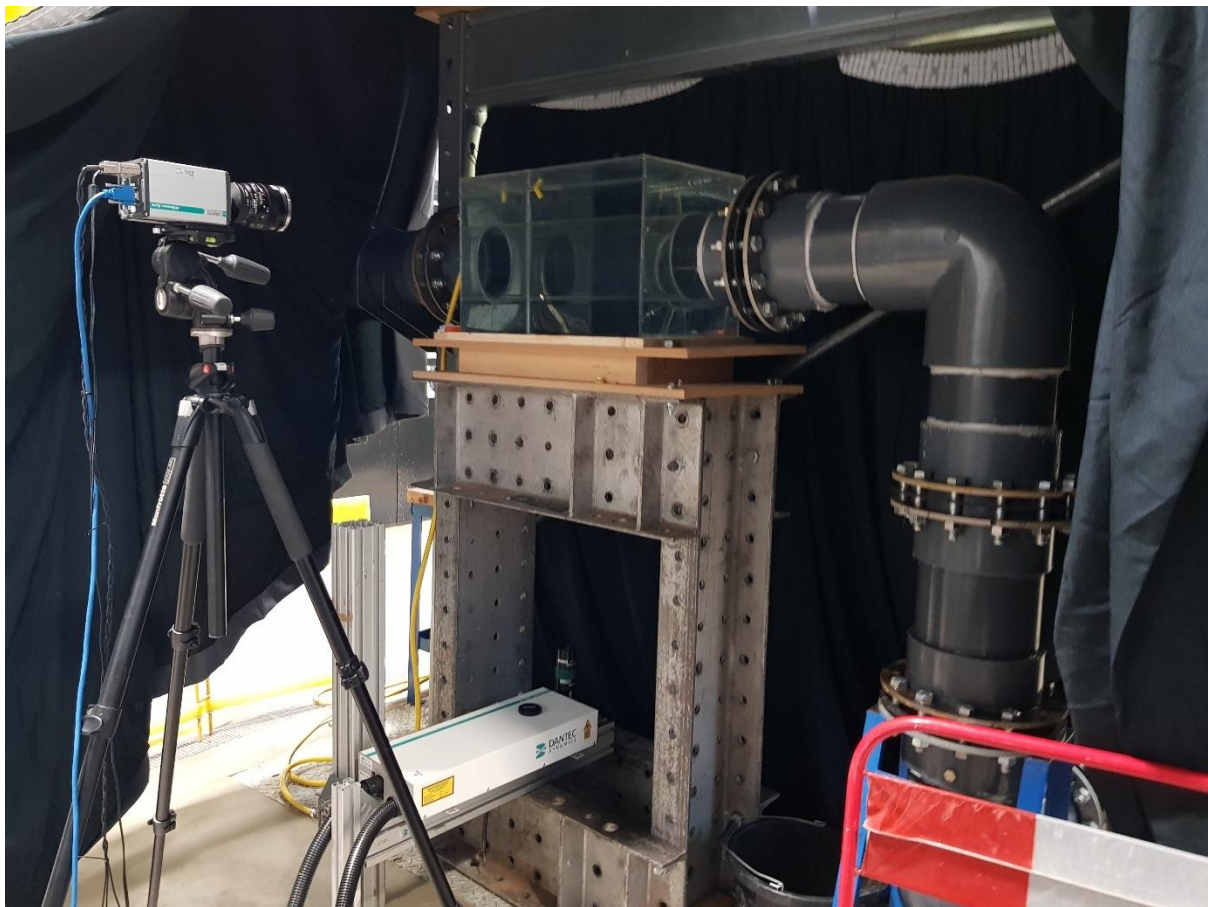
Figure 3-10: PIV experimental setup with camera and laser
