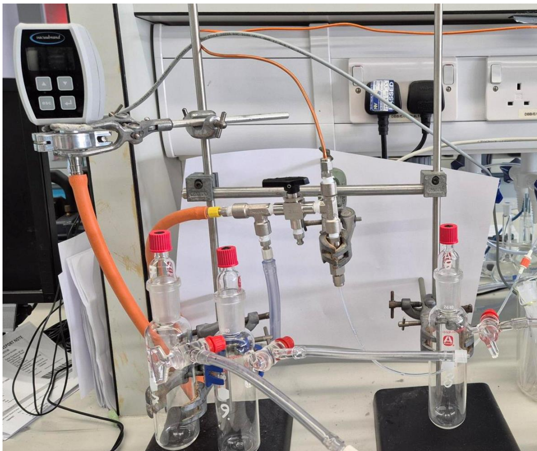
Figure 2.8 Experimental setup used for the batch screening of catalyst materials for DECO 2 R.
