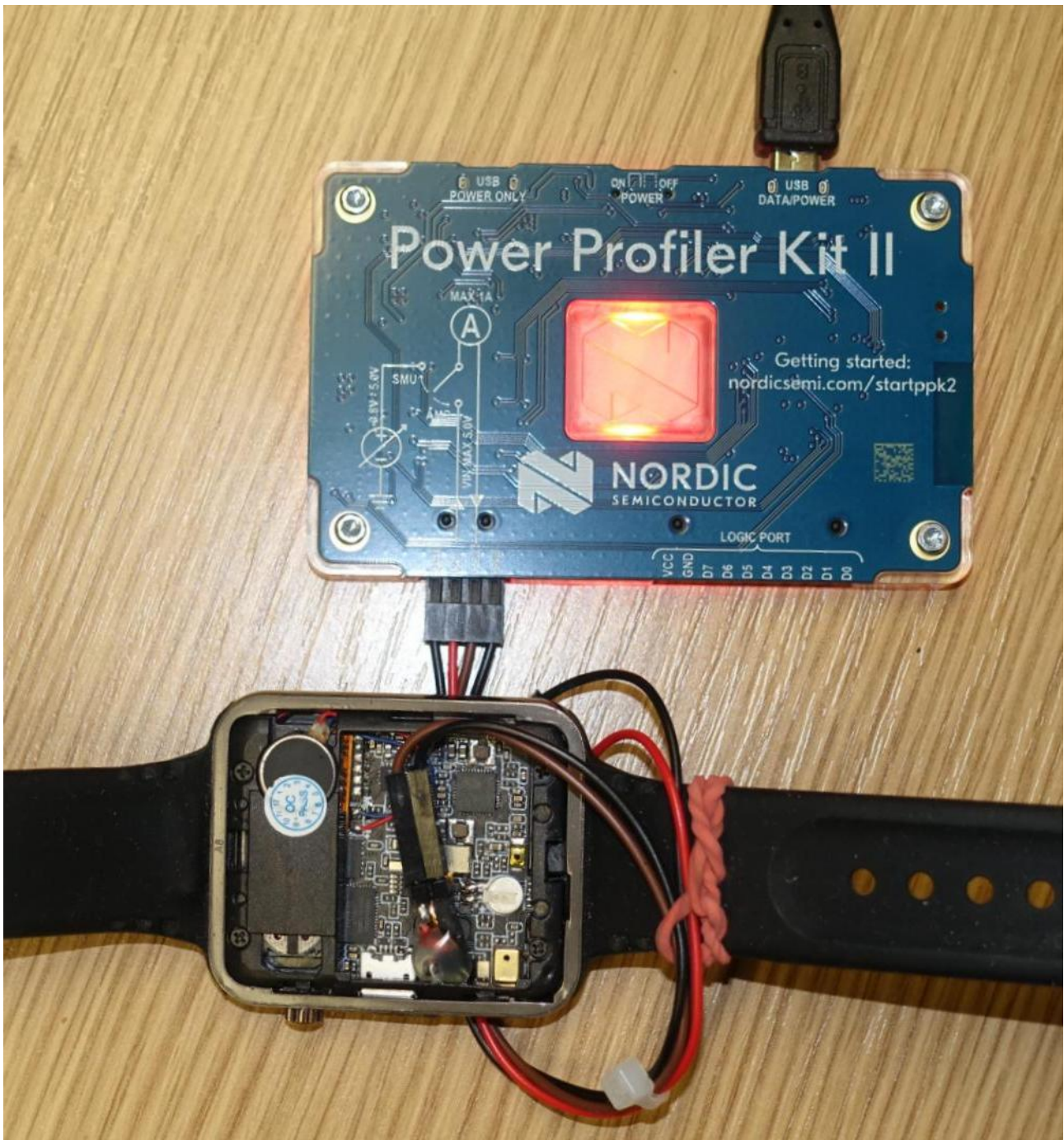
Figure 1: Power Profiler Kit II connected to Lilygo T-Watch S3. The red LED indicates that the PPK2 is powering the watch.
