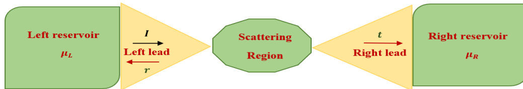
Figure 3. 1: A generic scattering region is connected to two ballistic leads with the chemical potentials \mu_L , and \mu_R , respectively, where r is the amplitude of the reflected wave due to an incoming wave from the left and t is the amplitude of the transmitted wave.
