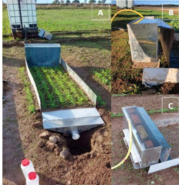
Figure 3.2 Photographs of overland flow simulations equipment where A shows the full set up, B shows the water flowing evenly out of the header tank and over the capillary matting, and C shows the header tank on the levelling platform with capillary matting held in place by bricks.
