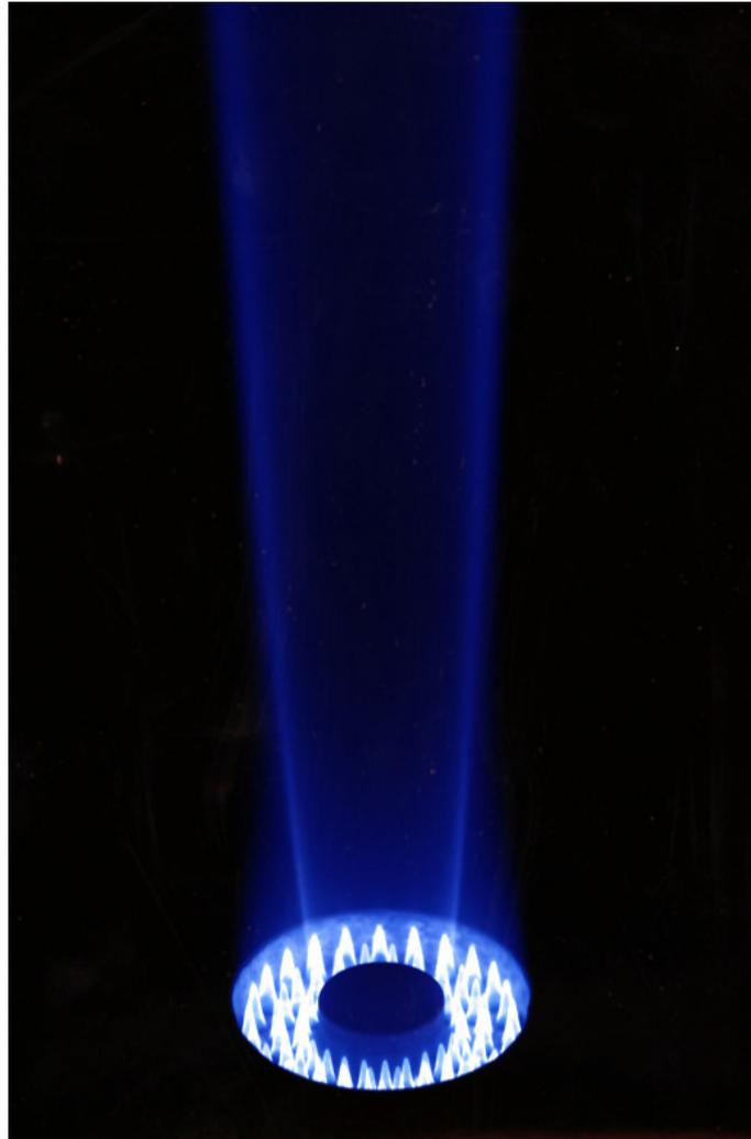
Figure 4.1: Picture of Sandia flame D taken from [7].
