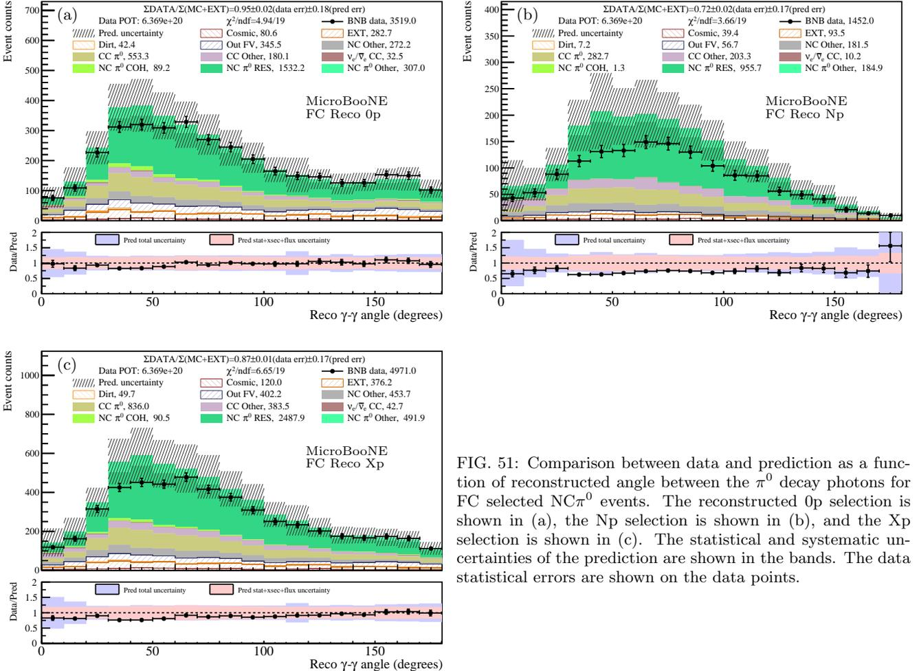
FIG. 51: Comparison between data and prediction as a function of reconstructed angle between the  $\pi^0$  decay photons for FC selected  $\text{NC}\pi^0$  events. The reconstructed 0p selection is shown in (a), the Np selection is shown in (b), and the Xp selection is shown in (c). The statistical and systematic uncertainties of the prediction are shown in the bands. The data statistical errors are shown on the data points.
