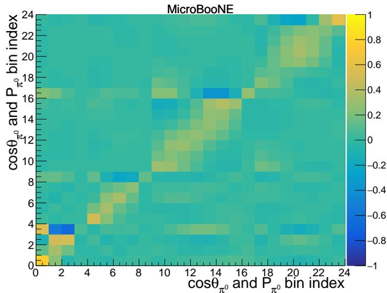
FIG. 20: The additional smearing matrix,  $A_C$ , obtained from the extraction of the the  $X_p \cos \theta_{\pi^0}$  and  $P_{\pi^0}$  differential cross section. The binning structure utilizes angle slices, which go from backwards on the left to forwards on the right. The true bins are those found in Sec. X and are the same as those for the extracted cross section.
