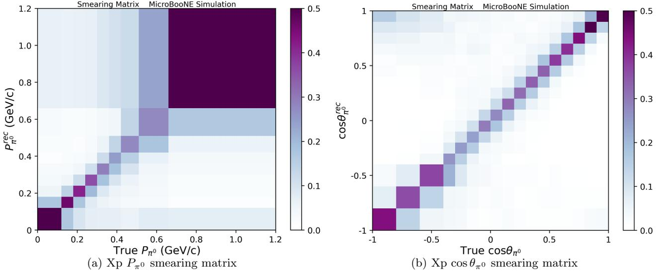
FIG. 7: Smearing matrices for the Xp (a) single-differential  $P_{\pi^0}$  and (b) single-differential  $\cos\theta_{\pi^0}$  measurements. Selected FC signal events are shown with each column normalized to one. In (a), the last bin corresponds to overflow in reconstructed space but ends at 1.2 GeV/c in truth space.
