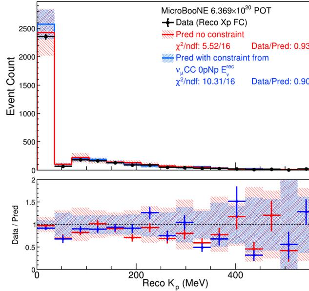
FIG. 26: Comparison between data and prediction as a function of reconstructed leading proton kinetic energy for the “tight” sideband. The last bin corresponds to overflow. The red (blue) lines and bands show the prediction without (with) the constraint. The constraint is from the  $\nu_{\mu}$ CC reconstructed neutrino energy distribution. The statistical and systematic uncertainties of the prediction are shown in the bands. The data statistical errors are shown on the data points.
