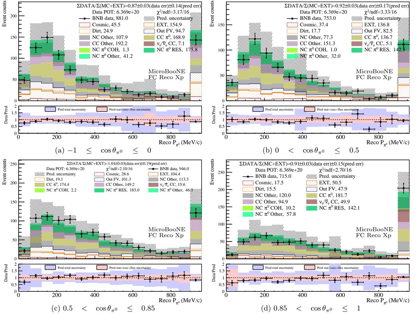
FIG. 23: Comparison between data and prediction as a function of reconstructed  $\pi^0$  momentum for the "tight" Xp sideband. Different  $\cos \theta_{\pi^0}$  slices are shown in each subplot. The last bin in each slice corresponds to momentum overflow. The statistical and systematic uncertainties of the prediction are shown in the bands. The data statistical errors are shown on the data points.
