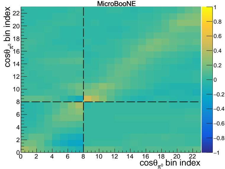
FIG. 17: The additional smearing matrix,  $A_C$ , obtained from the simultaneous extraction of the the 0p and Np  $\cos\theta_{\pi^0}$  differential cross section. The dashed lines separate the 0p and Np channels. The true bins are those found in Sec. X and are the same as those for the extracted cross section.
