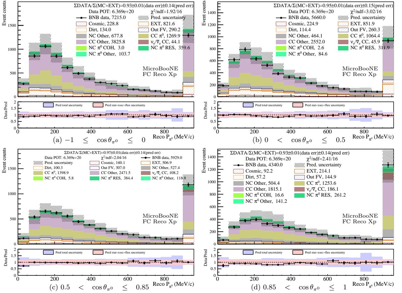
FIG. 32: Comparison between data and prediction as a function of reconstructed  $\pi^0$  momentum for the "loose" Xp sideband. Different  $\cos \theta_{\pi^0}$  slices are shown in each subplot. The last bin in each slice corresponds to momentum overflow. The statistical and systematic uncertainties of the prediction are shown in the bands. The data statistical errors are shown on the data points.
