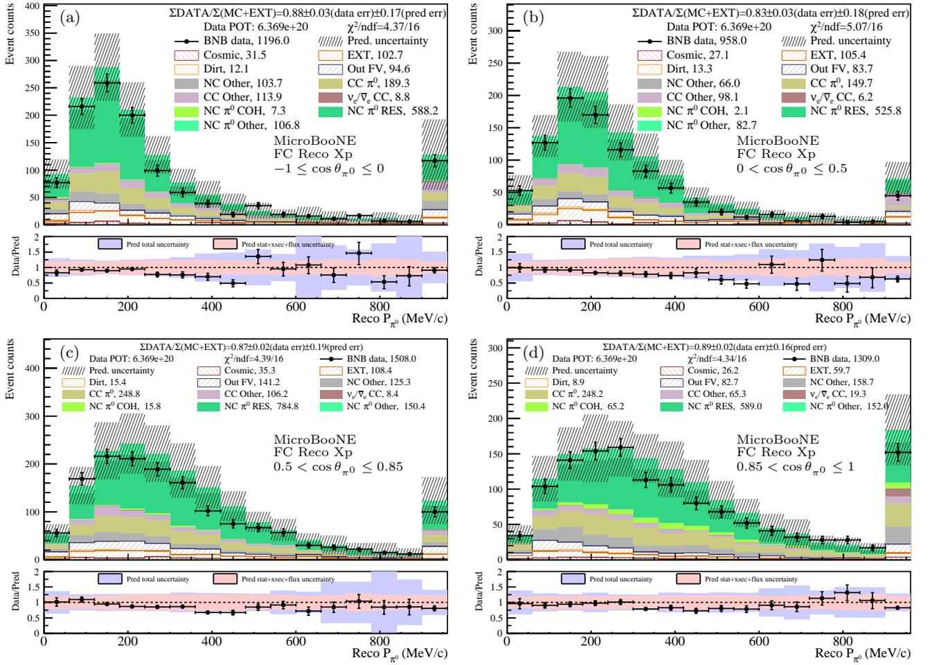
FIG. 41: Comparison between data and prediction as a function of reconstructed  $\pi^0$  momentum for FC selected NC  $\pi^0$  Xp events. Different  $\cos \theta_{\pi^0}$  slices are shown in each subfigure. The last bin in each slice corresponds to overflow. The statistical and systematic uncertainties of the prediction are shown in the bands. The data statistical errors are shown on the data points.
