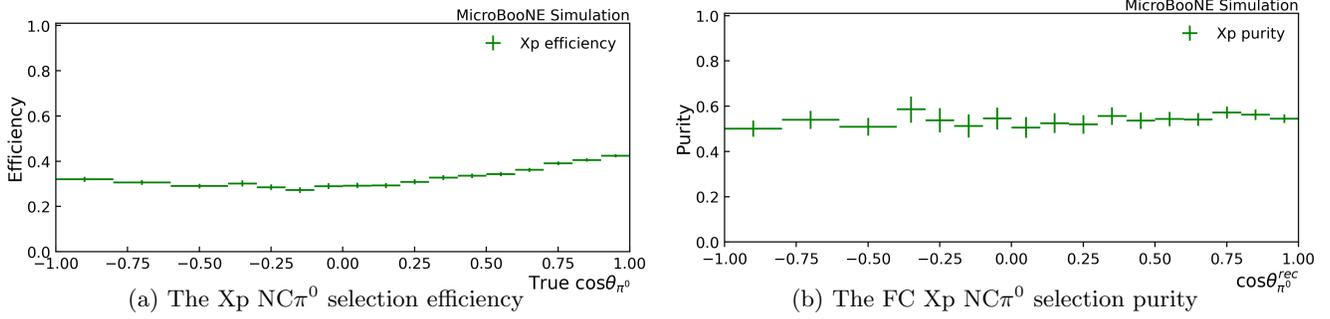
FIG. 5: (a) The Xp NC $\pi^0$  selection efficiency as a function of true  $\cos\theta_{\pi^0}$ . (b) The Xp NC $\pi^0$  selection purity as a function of reconstructed  $\cos\theta_{\pi^0}$  for FC events. The error bars contain only statistical uncertainty.
