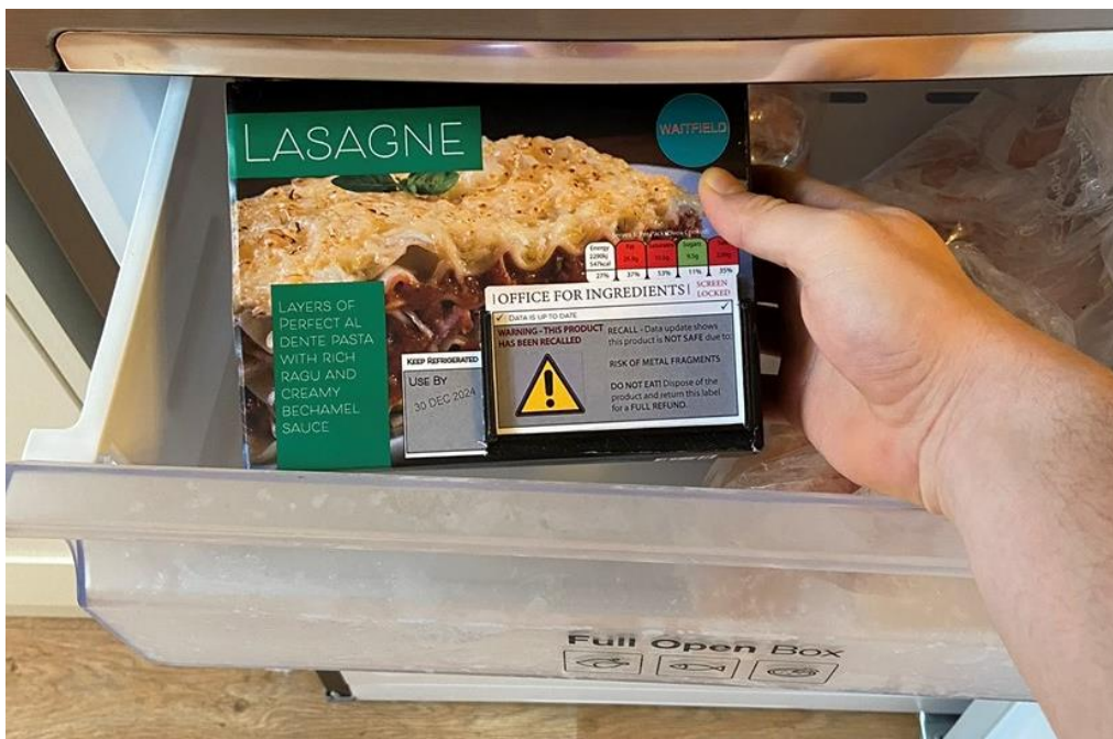
Figure 26. Smart packaging for a supermarket ready meal. The display cycles through information updated via the Internet, similar to modern digital price tag displays.
