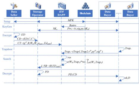
Fig. 4. Data circulation process based on attribute-based searchable encryption.
