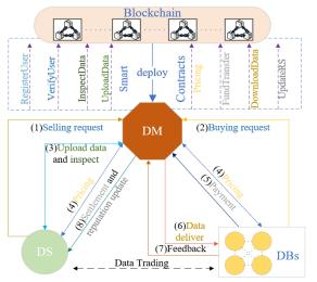
Fig. 3. Data trading process and corresponding smart contracts deployed on the blockchain.
