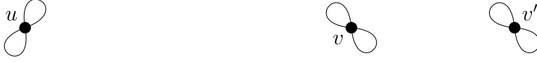
Figure 5.10: The base graphs, left (\mathcal{P}_1, \phi_0) and right (\mathcal{P}_2, \phi_2) , for C_2 -symmetric linearly constrained frameworks.
