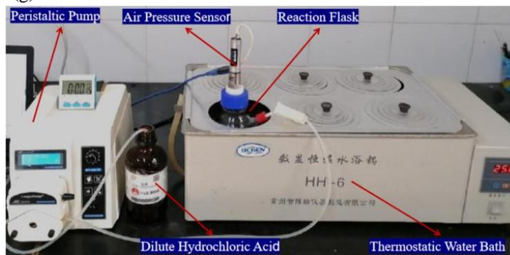
**Fig. 6.** Micro-precision digital carbonation measuring instrument.
