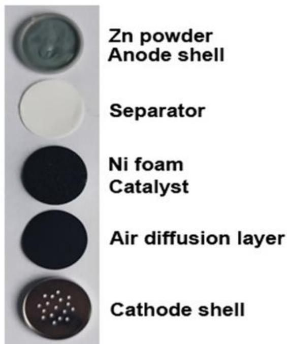
**Figure S30** Photograph of the zinc-air button cell components.
