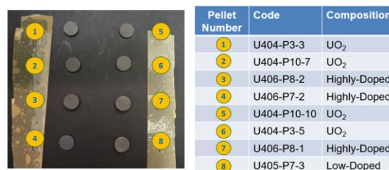
Fig. 1. Pellets used in the experiments: (a) RGB image of the eight pellets for reference, and (b) description of each pellet.
