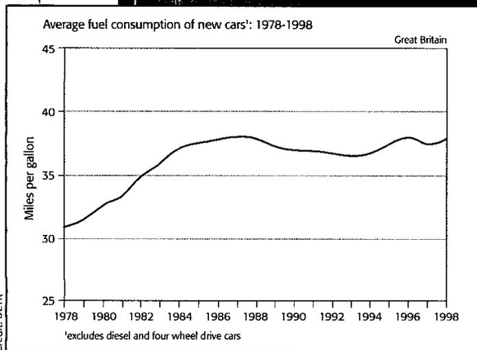
Fig 2: Car fuel efficiency has remained static since the late 1980s
