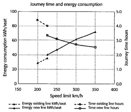
Fig 3: Energy consumption in trains rises dramatically at speeds of more than 200km/h. Solid lines represent journey time and energy consumption on a new track, broken lines show extrapolations for lower speed operation on the existing line
