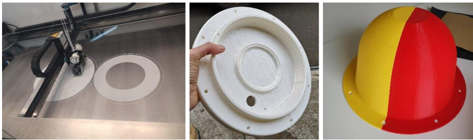
Fig. 3. From left to right: Base and dome being manufactured on the Builder Extreme 2000 Pro; Final base component former; Final dome component with MEX halves bonded together
