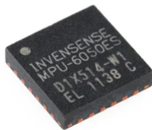
Figure 23 – 6-Axis Gyro/Accelerometer IC – MPU-6050 (SparkFun, 2021)
