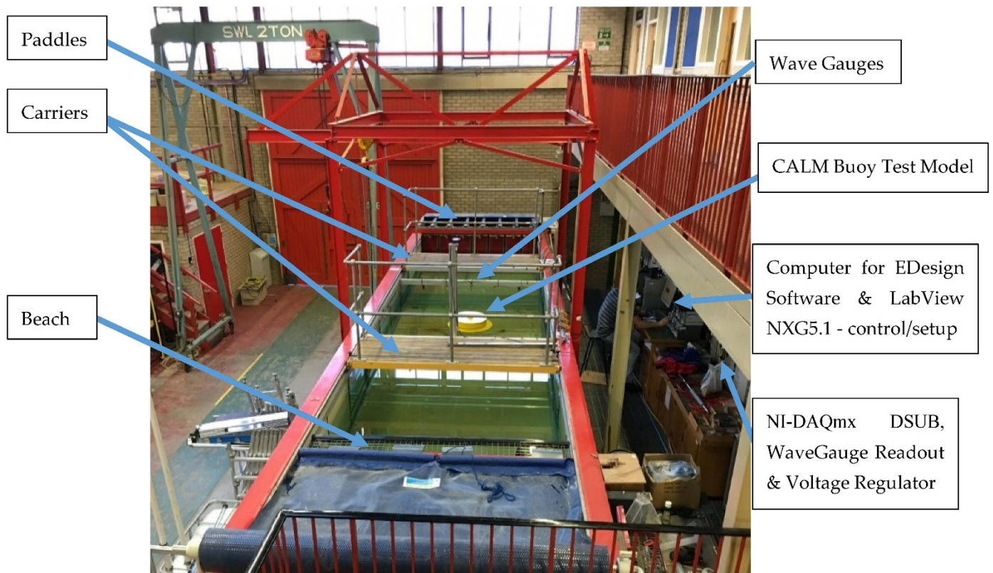
Figure 3. Test basin at the Lancaster University Wave Tank facility showing the location of the buoy and wave gauges used in the experiment.
