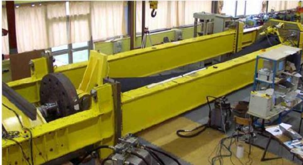
Figure 18 Combined bending fatigue + tension using a test bench (Courtesy: Rampi et al. 2006)
