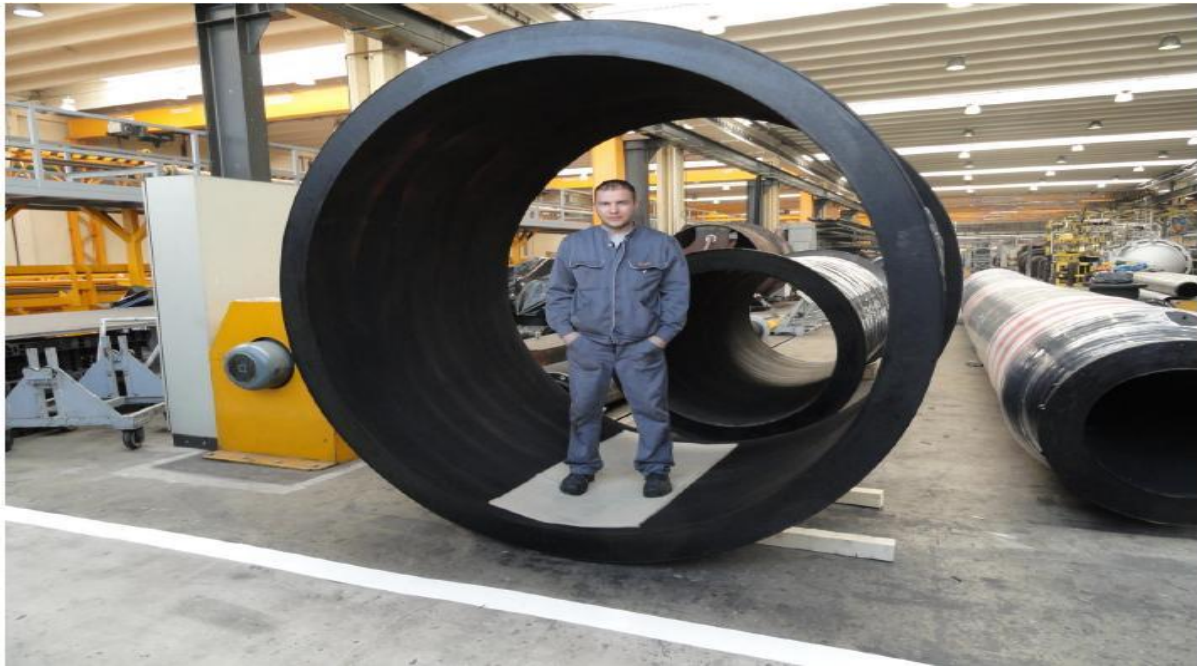
Figure 2 The extreme size of dredging hoses compared to floating hoses (Courtesy: Antal S. et al. 2012; Adapted with permission of Germa Hornsby of Continental Dunlop Oil & Marine).
