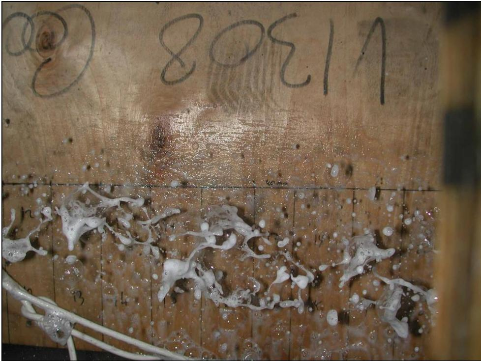
**Figure 5:9 Large air gaps visible within jet (Taken approximately 80 cm from end of branchpipe)**
