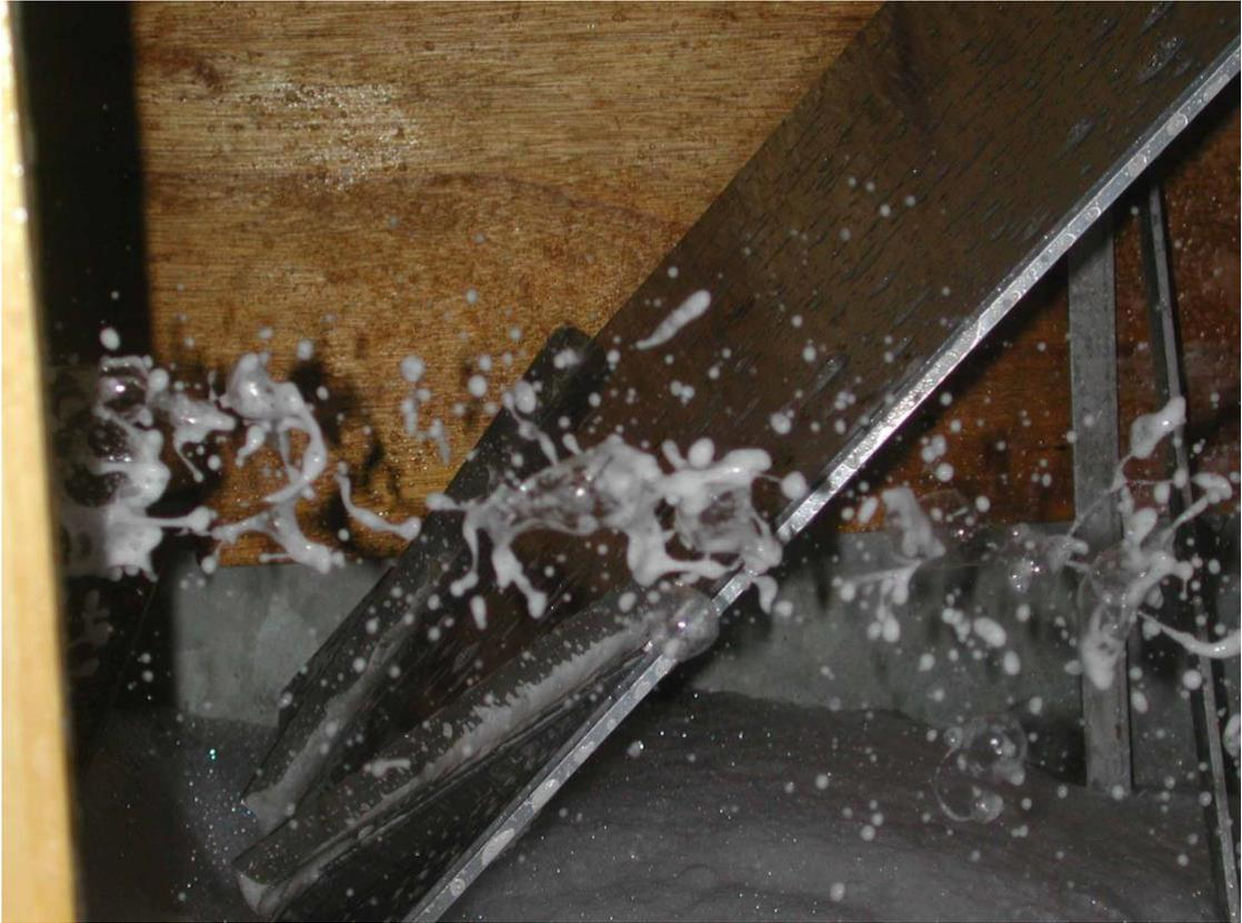
**Figure 5:10 Bubbles in flight (large bubbles approx. 25 mm diameter)**
