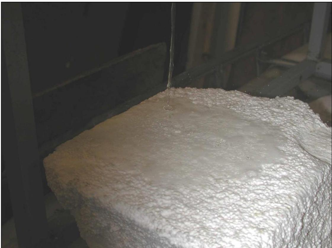
**Figure 6:6 Jet impinging on rough surface**
