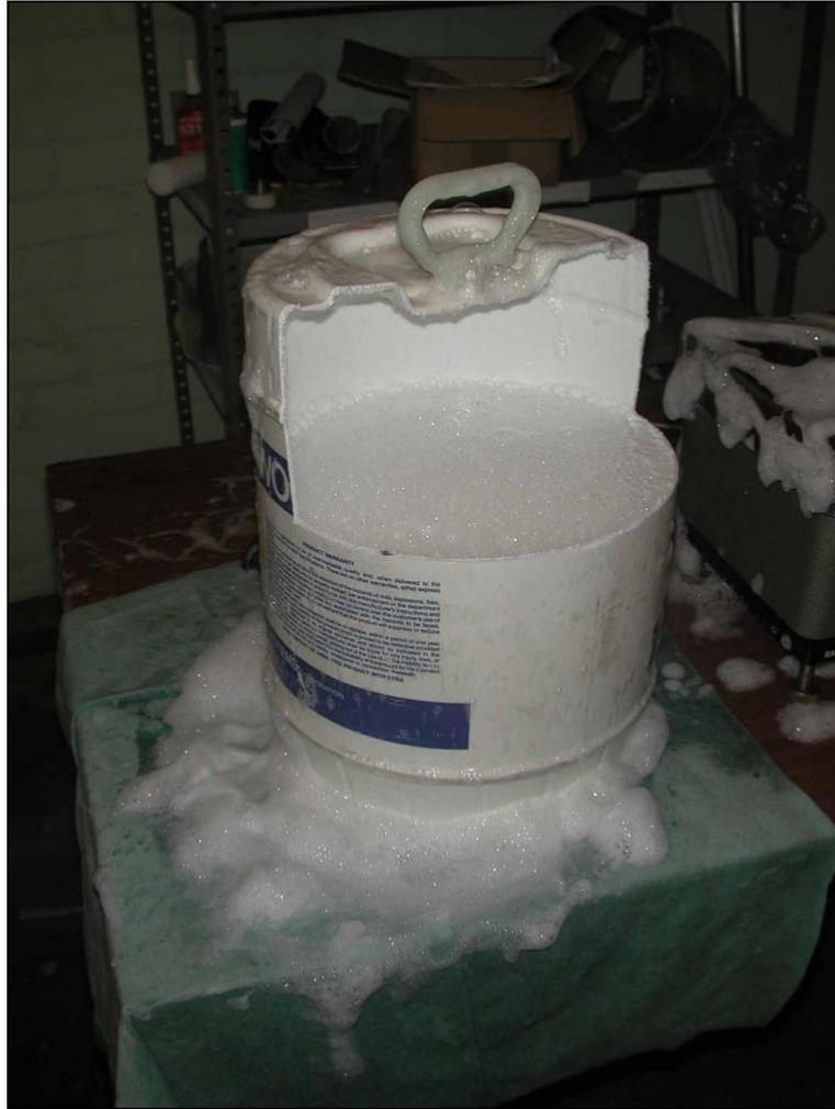
**Figure 3:10** Photo of larger foam collecting vessel
