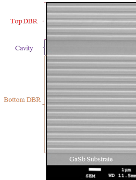
Fig. S1. An SEM image of the RCLED structure after epitaxial growth, showing the DBR mirrors and microcavity
