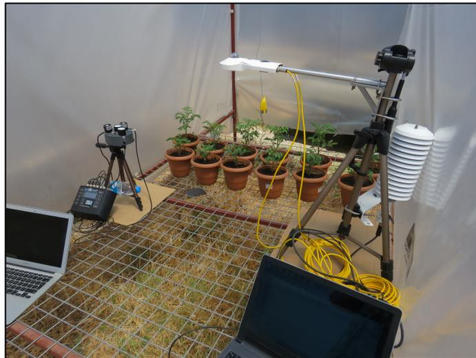
**Figure 7.2:** The inside of a polytunnel showing the internal metallic mesh bench, the Skye radiation sensors (left hand side) and the CNR4 net radiometer (right hand side).
