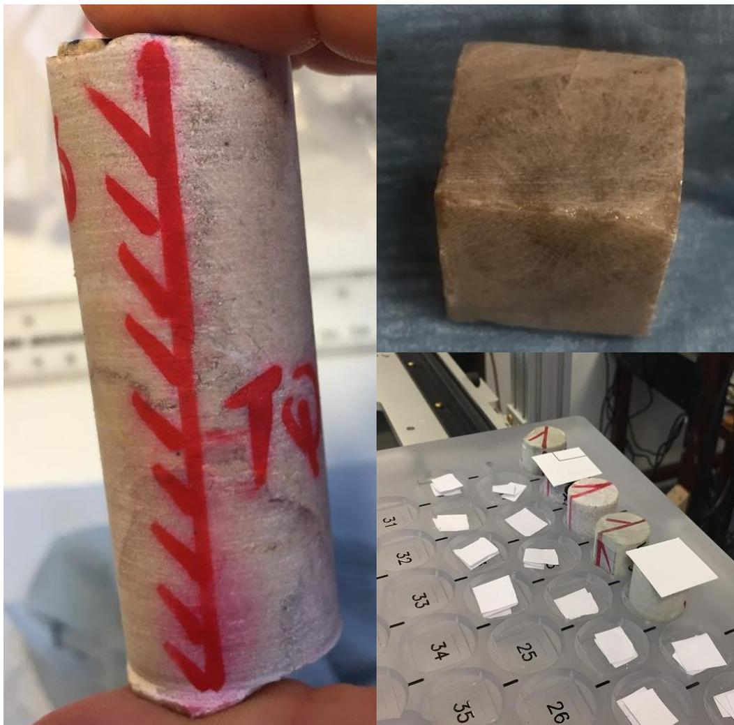
**Figure 34** On the left side is plug of length 5 cm, coming as a result of the drilling process. This plug is cut for smaller pieces, in order to get a final sample. On top right is a cube sample, this type of samples is achieved by the direct cutting on a rock saw. The dimensions are 2,5x2,5x2,5 cm. This method is used for samples which are fractured or having any other defect and cannot be drilled. Bottom right, picture of Rapid 2G sample table.
