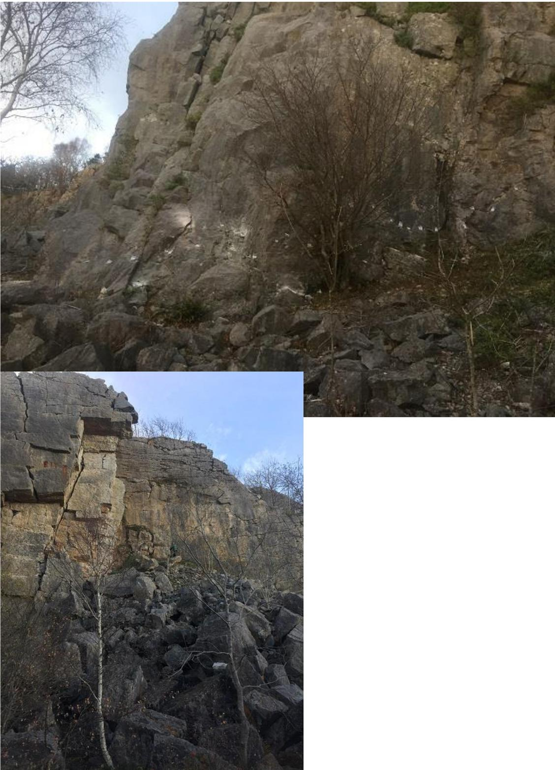
**Figure 32** On top can be seen a density of sampling in the quarries. Each small white spot is approx. 25 cm from each other, there was the susceptibility sample taken from. Big white spot is hand sample for paleomagnetic measurements. Those are 1 m from each other.
