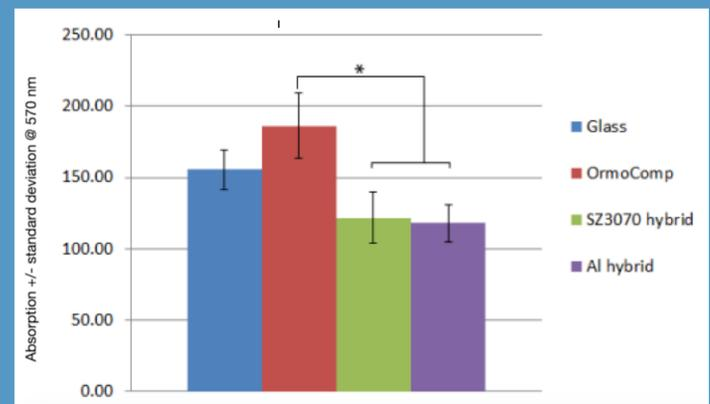
MTT assay was performed on NIH 3T3 fibroblasts grown on spin-coated and UV- cured hybrid polymer films. Results are presented as absorption +/- standard deviation, n = 16. Commonly used Zr- based hybrid material, SZ3070 (previously shown to be as biocompatible as a surgical suture [4]) was shown to be as biocompatible as the Al hybrid. Commercially available OrmoComp was shown to be the most biocompatible *in vitro*.
