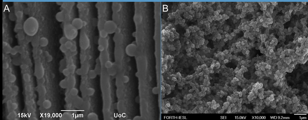
A – lines fabricated using 2 mm/s writing speed and 40X 0.8 NA objective lens. Nanoparticles can be seen on the polymer surface. B – a SEM micrograph of uncrosslinked Al-hybrid. The material shows a nanoparticle-based texture.
