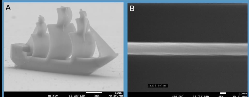
A - 3D structures with fine features can be fabricated. B - suspended lines with down to 200 nm can be fabricated. Both structures were fabricated using 40 % (20 mW) laser power and 10 mm/s scanning speed out of 1:1:2 material using a 63x oil immersion objective lens.
