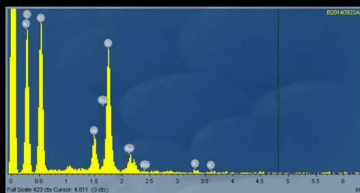
The presence of aluminium was supported by EDS spectra. XRD measurements show crystals of aluminium oxide present in the material (data not presented).
