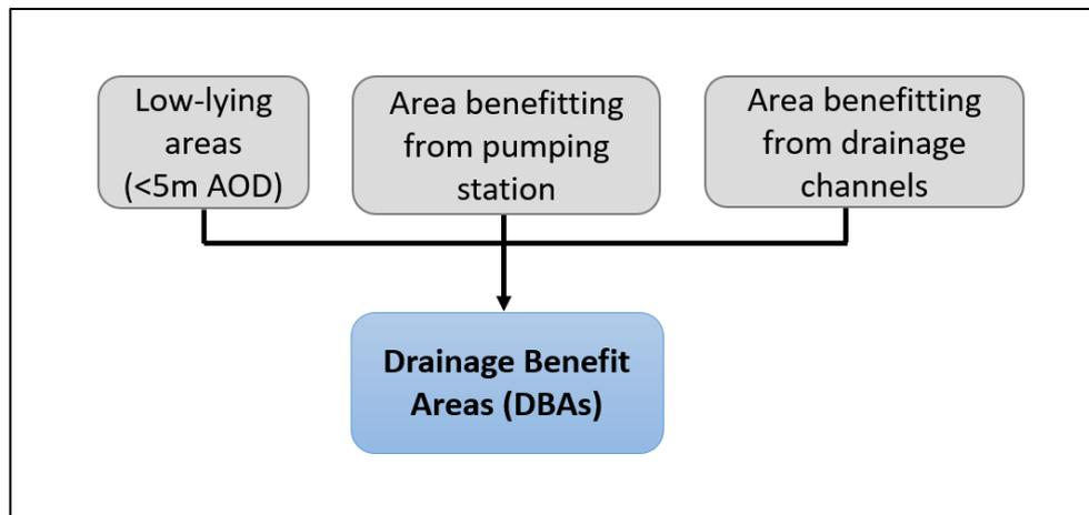
Figure 11: Basic criteria in determining drainage benefit areas.
