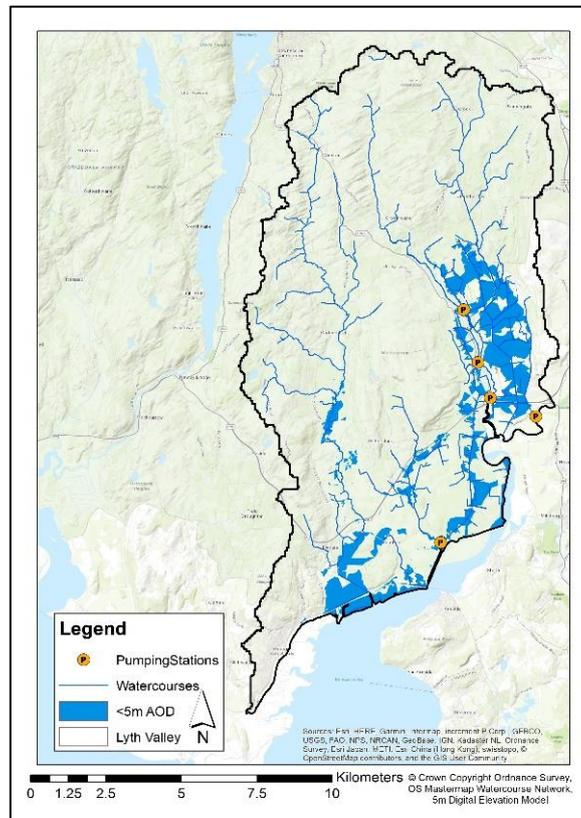
**Figure 13:** The location of each of the 5 pumping stations within Lyth Valley (right), with reference to the presence of low-lying land and watercourses.
