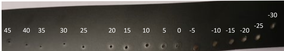
Figure 5: Effects of varying the neutral position of the lens by 5% from 45% to -30%
