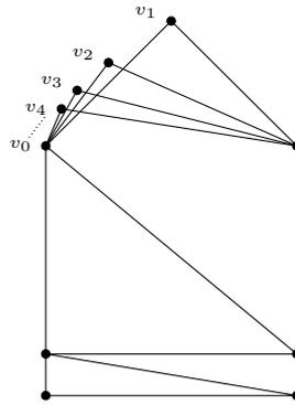
Fig. 4.2 An infinitesimally flexible independent framework  $(G, p)$  in the Euclidean plane that is continuously rigid. The sequence  $\{p_{v_1}, p_{v_2}, \dots\}$  converges to  $p_{v_0}$ . We may choose  $p_{v_0}, p_{v_1}, p_{v_2}, \dots$  so as to be an algebraically independent set, thus we can assume  $(G, p)$  is also generic.
