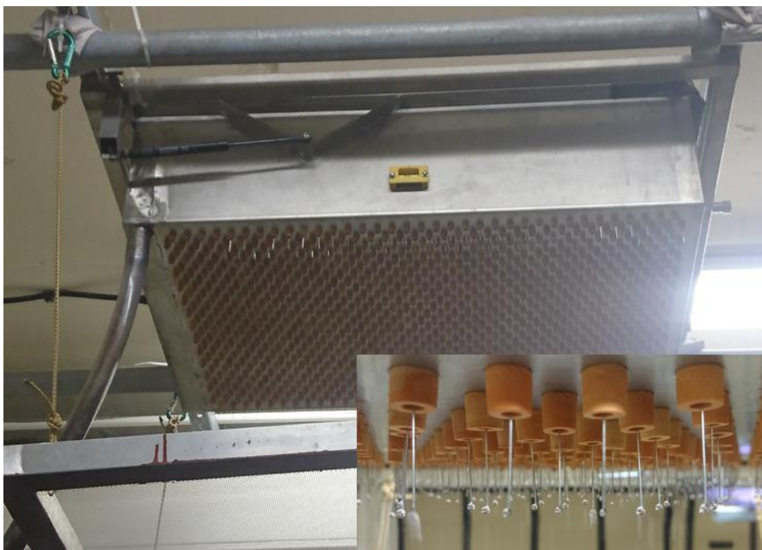
Figure 4.2. Gravity-fed rainfall simulator and the mesh hanging below with a close up of the droplets on the needle points.
