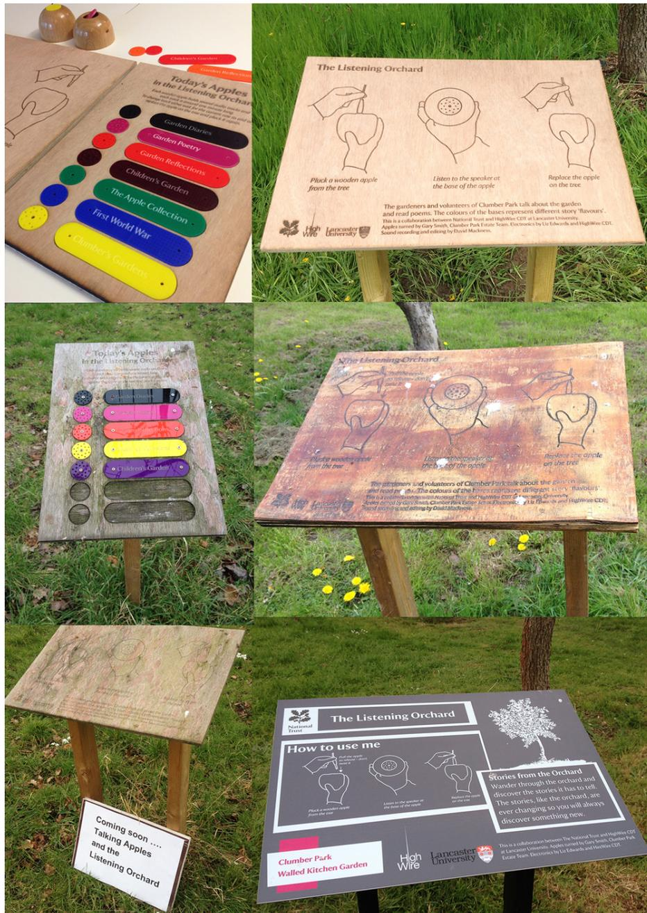
**Figure 5.26:** Signage: Earlier designs met design criteria set by design framework but weathered rapidly. New signage was developed by the Gardens Team as they took ownership of the installation
