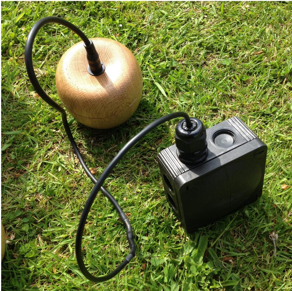
**Figure 5.25:** Audio Apple with charging pack. Every night the apples were put on charge and every morning they were put back in the Listening Orchard, creating additional work for the team.
