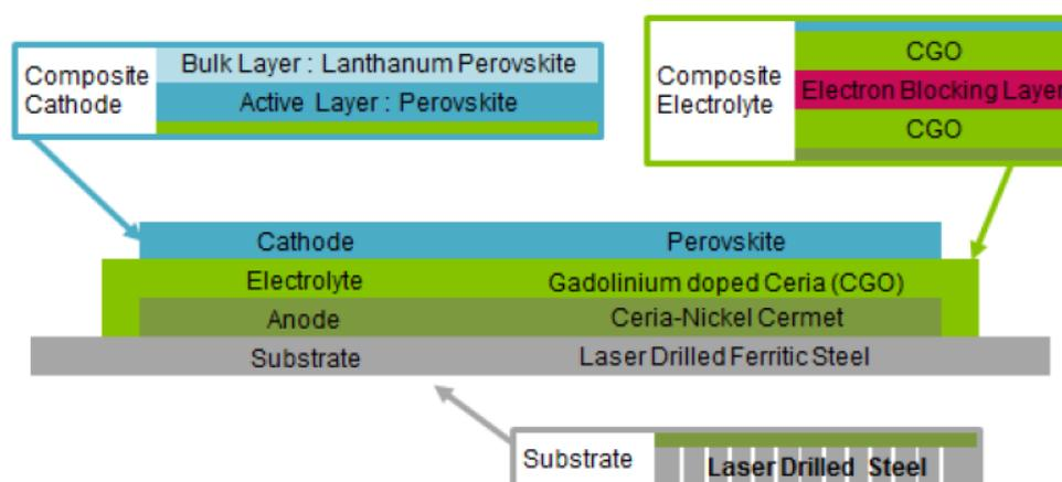
Figure 1 Schematic representation of a Ceres Power SteelCell™.
