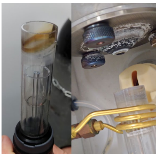
Figure 4.10 Damage on torch and precipitates on ICP-OES components after 5 hours of continuous operation with 1 M KOH matrix.
