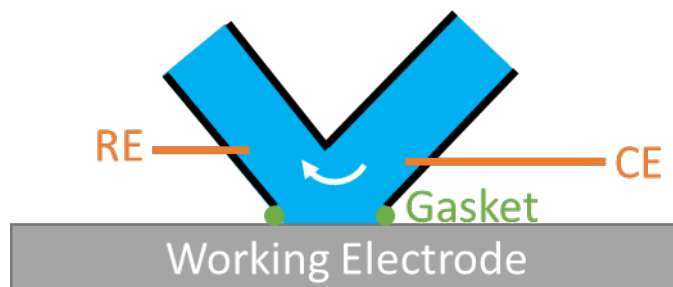
Figure 2.4 A schematic of the v-channel scanning droplet cell. CE = counter electrode, RE = reference electrode. White arrow represents the path of the electrolyte flow.
