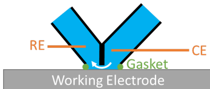
Figure 2.5 A schematic of the modified scanning droplet cell. CE = counter electrode, RE = reference electrode. White arrow represents the path of the electrolyte flow.
