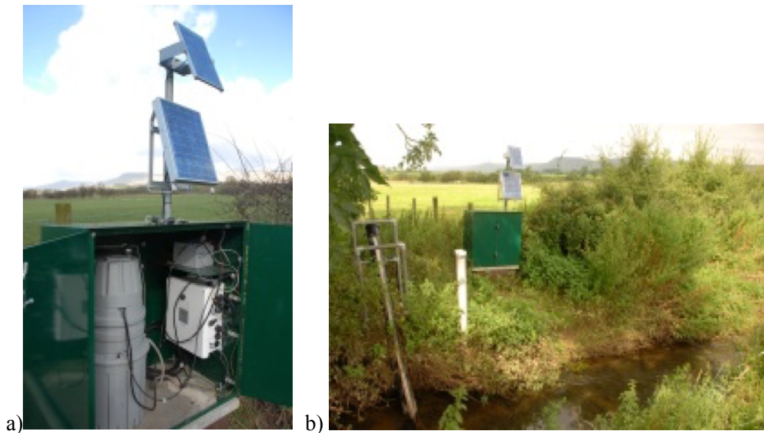
Figure 3-3 - a) The WISER water quality monitoring system at the main weir, Blind Beck Experimental Catchment, Cumbria, UK, b) The water-level recorder (left) and WISER water quality monitoring system (centre) at the main weir, Blind Beck Experimental Catchment, Cumbria, UK (Photos courtesy of: NA Chappell)
