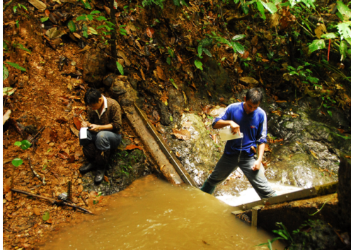
a) Preparing to collect a water sample (for suspended sediment determination) at the main station of the Baru Experimental Catchment, Sabah, Malaysian Borneo
