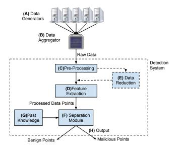
Fig. 2. Generalised architecture of C&C detection systems
